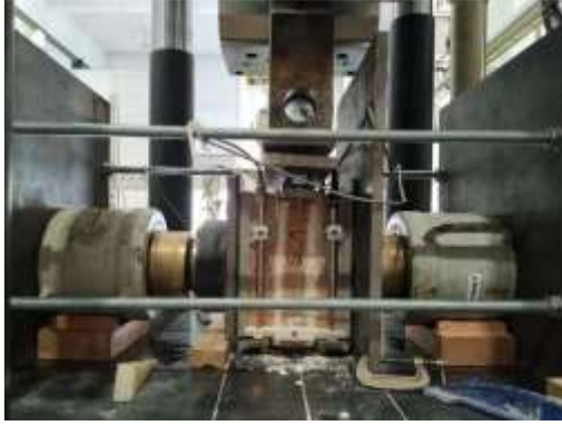
Figure 6. Experimental setup for the application of triplet shear tests to fired brick masonry specimens. (adapted from (Bianchini et al., 2023a))
