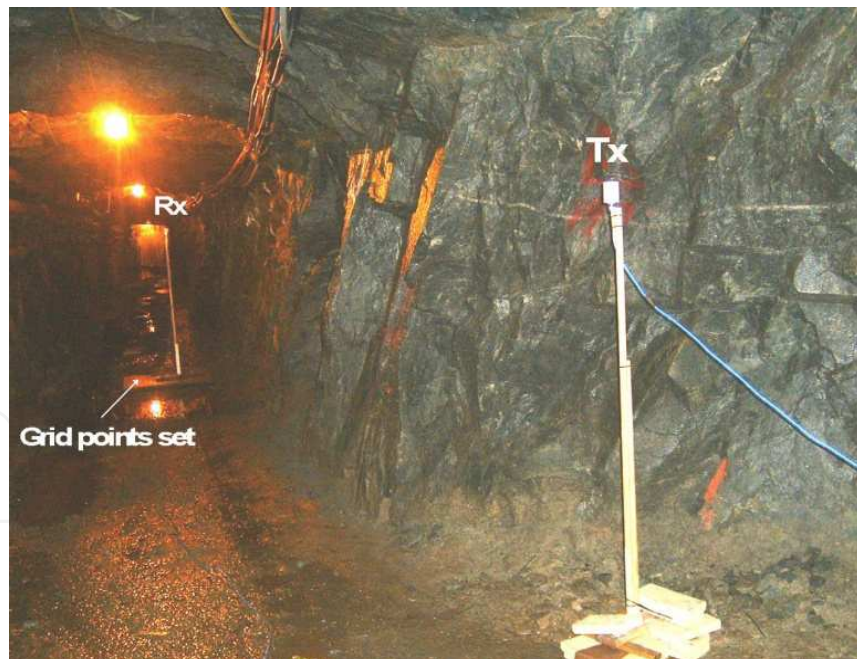
Fig. 1. Photography of the Underground Gallery and the Measurement Arrangement.
