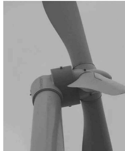
Fig. 1. Photo of a 1.5-MW direct-drive wind turbine with permanent-magnet generator of Zephyros. Source: Zephyros BV.
