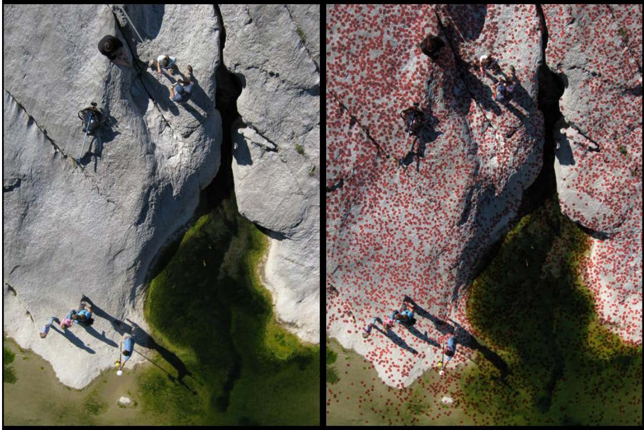
Figure 6. A close-up image taken with the helikite (left) and the same image overlaid with red topographic points derived using SfM (right). Even some submerged areas produce valid topographic points, as long as they are clear and have some spatial texture. In these frames such points are red, but cover the greenish-colored submerged bed.
