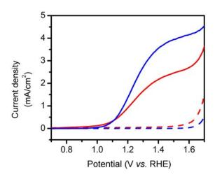
**Figure 1 | Photoelectrochemical response of nanostructured hematite electrodes.** The plot displays the photocurrent (solid lines) and dark current (dashed lines) for the 2L (red) and 6L (blue) electrodes.
