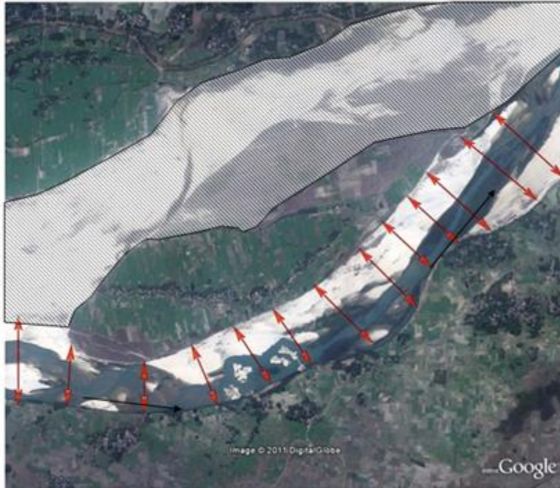
Fig. 9 Representation of an island in the Damodar River within LISFLOOD-FP. Red arrows show the 1D configuration of the main channel. The shallower secondary channel and the floodplain, depicted with shading, are handled by the 2D component of the model.
