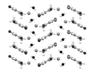
Figure 3 Packing of the ionic cocrystals (H<sub>2</sub>ba)·(KBr)·(H<sub>2</sub>O)<sub>2</sub>.
