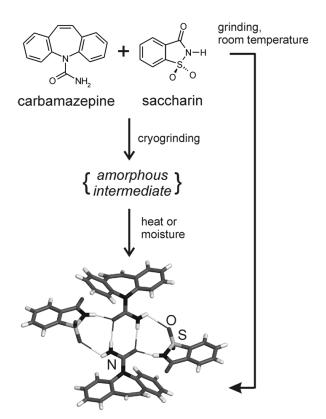
**Figure 7** Mechanochemical cocrystallization by neat grinding of carbamazepine and saccharin, [31, 173] involving an amorphous intermediate.
