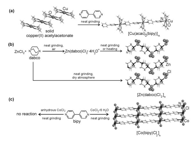
**Figure 12** (a) Mechanochemical construction of a 1-D coordination polymer from copper(II) acetylacetonate and bipy; <sup>[39]</sup> (b) formation of the coordination polymer ZnCl<sub>2</sub>(dabco) by manual grinding in air and grinding in a dry atmosphere; <sup>[279]</sup> and (c) difference in mechanochemical reactivity of bipy towards anhydrous CoCl<sub>2</sub> and CoCl<sub>2</sub>·6H<sub>2</sub>O. <sup>[280]</sup>
