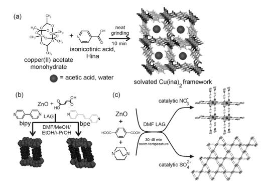
**Figure 16** Mechanochemical synthesis of porous MOFs: (a) by neat grinding; <sup>[40]</sup> (b) by liquid-assisted grinding <sup>[294]</sup> and by ion- and liquid-assisted grinding, exploiting the catalytic effect of nitrates and sulfates. <sup>[295]</sup>
