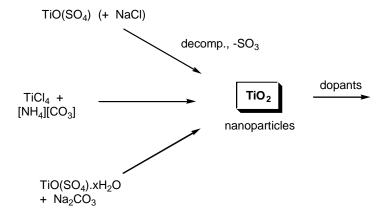
Scheme 2 General ball milling routes to metal oxides.
