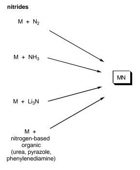
**Scheme 3** General ball milling routes to halides, sulfides and nitrides.
