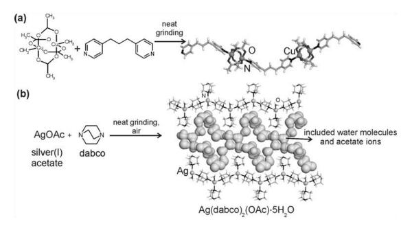
**Figure 14** (a) Mechanochemical construction of a 1-D coordination polymer by ligand exchange on the copper(II) acetate paddlewheel complex; [283] (b) formation of a hydrated coordination polymer by neat manual grinding of silver(I) acetate and dabco in air. Water and acetate guests are shown using the space-filling model. [279]
