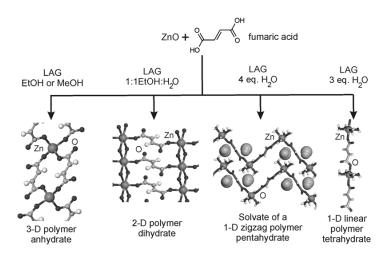
Figure 15 Screening for coordination polymers from ZnO using LAG. [290]
