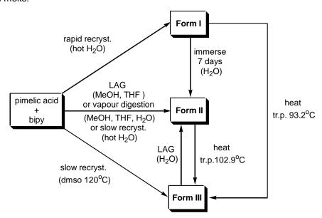
**Scheme 5** Preparation and transformation conditions of the three crystal forms of (bipy)·(H<sub>2</sub>pma) (tr.p.: transition point).
