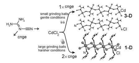
**Figure 13** The ligand cnge with different metal binding sites indicated by arrows and its reactions with CdCl<sub>2</sub> upon neat grinding under various reaction conditions.
