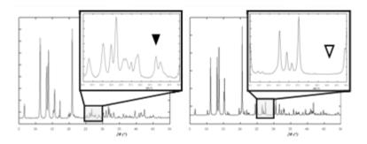
**Figure 19** An example of comparison between the experimental powder XRD pattern of a material prepared by mechanochemical synthesis (left) with the simulated powder XRD pattern of a potential candidate of known structure prepared previously by a solvothermal route (right). Adapted from ref. 306, permission to be sought.
