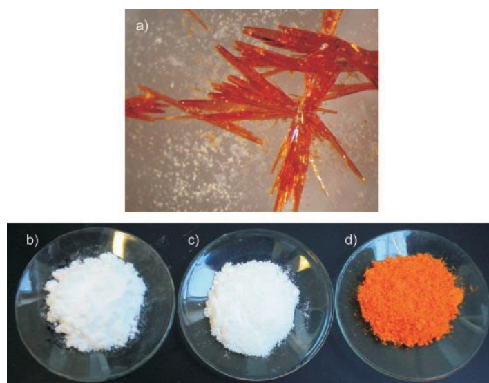
Figure 7 A coloured co-crystal formed from white component solids: (a) single crystals of the 1:1 acetaminophen and 2,4-pyridine dicarboxylic acid co-crystal, (b) powdered acetaminophen, (c) powdered 2,4-pyridine dicarboxylic acid, and (d) powdered co-crystal (reproduced with permission from ref. (49)).
