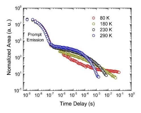
Figure 2. Time resolved fluorescence decay of DDMA-TXO2 in zeonex matrix.
