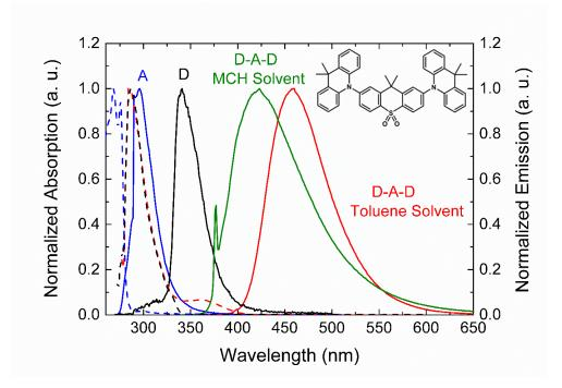
**Figure 1**. Normalized absorption and emission spectra of acceptor (A), donor (D), and D-A-D (DDMA-TXO2) molecules. Donor unit is diluted in toluene solvent, acceptor unit in MCH solvent and D-A-D in both solvents. The acceptor and donor units were excited at 266 nm and the D-A-D at 337 nm. Inset graph shows the chemical structure of DDMA-TXO2.
