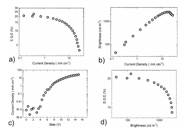
**Figure 7.** a) E.Q.E. *versus* current density b) brightness *versus* current density c) current density *versus* bias and d) E.Q.E. *versus* brightness curves for DDMA-TXO2:DPEPO devices.
