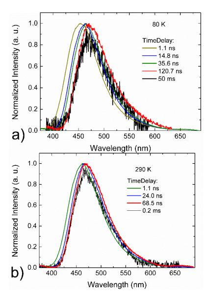
**Figure 5.** Time resolved normalized emission spectra of DDMA-TXO2 in DPEPO matrix at a) 80 K and b) 290 K.
