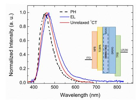
**Figure 6.** Phosphorescence (PH), eletroluminescence (EL) and unrelaxed <sup>1</sup>CT spectra. Inset figure architecture of the optimized DDMA-TXO2:DPEPO device.
