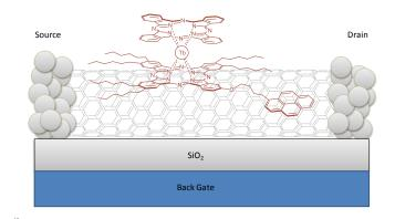
Fig. 20 A totally schematic view of a supramolecular spin valve device based on an asymmetric double decker terbium(III) bis phthalocyanine physisorbed onto a single walled carbon nanotube. In the actual device, about 100 nm separates source and drain electrodes and multiple molecules can physisorb to the tube.
