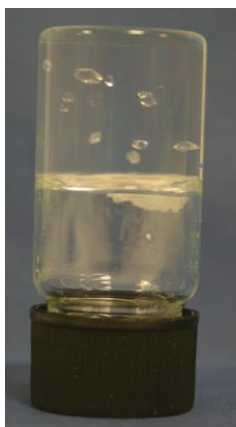
Figure 5. Crystals of Form III carbamazepine growing in a supramolecular organogel (reproduced with permission from reference 44).
