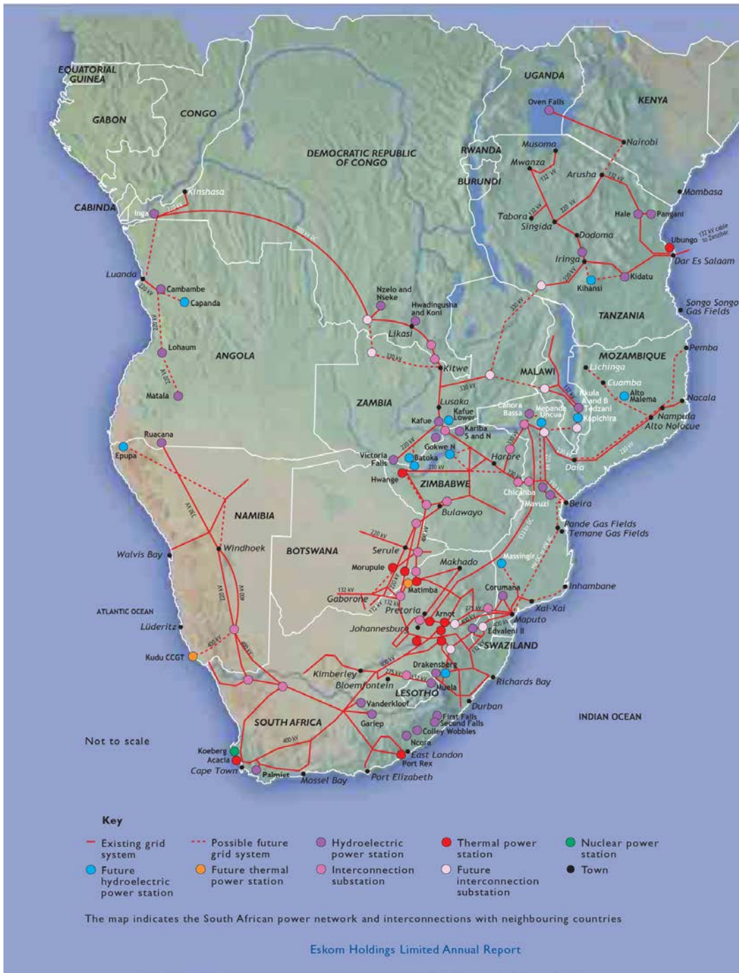
Figure 2: South African electricity grid network, managed by Eskom Source: www.geni.org (Global Energy Network Institute)
