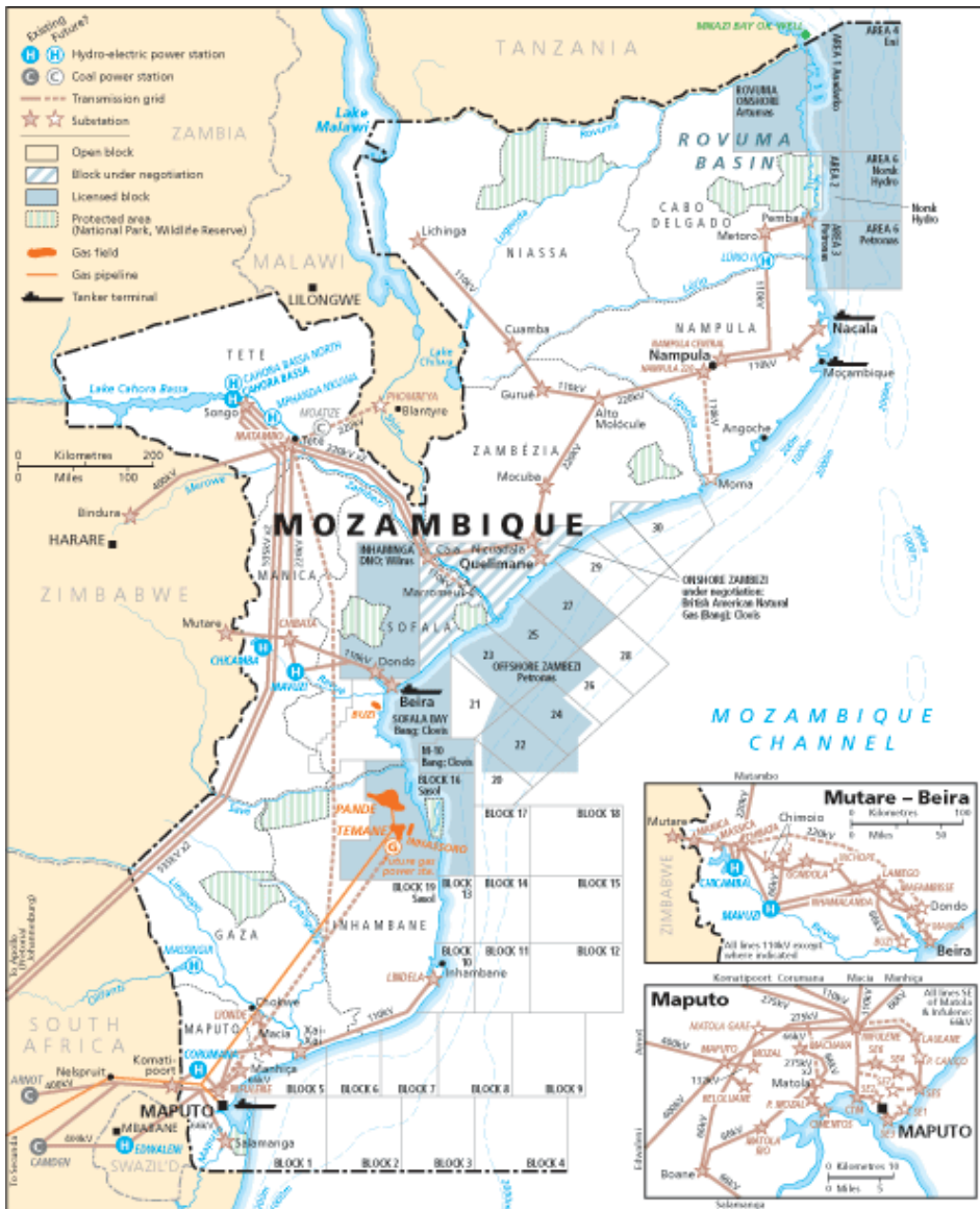
Figure 1: Mozambican electricity grid network, managed by Electricidade de Moçambique (EDM) Source: www.geni.org (Global Energy Network Institute)
