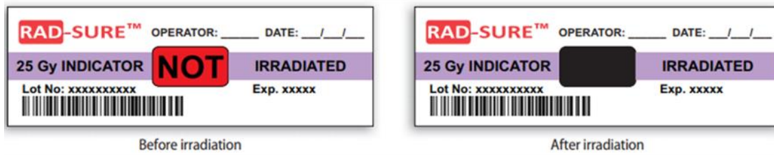
Figure 42. Radiochromic film labels used for irradiation detection on blood bags. Figure reproduced from reference 164.
