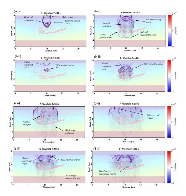
Figure 2: Snapshots of seismic wave propagation for 'Shot 1' (yellow star) after 0.80 (a), 1.30 (b), 1.80 (c) and 2.30 (d) seconds for the P- (i) and S- (ii) wavefield.
