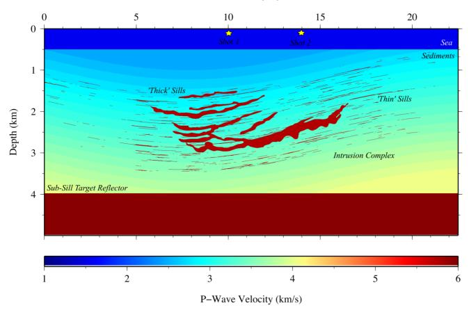
Figure 1: P-wave velocity model containing both seismically resolvable 'thick' sills taken from the interpreted seismic data, and unresolvable 'thin' sills. Two shot locations are presented here, 'Shot 1' at 10 km and 'Shot 2' at 14 km.
