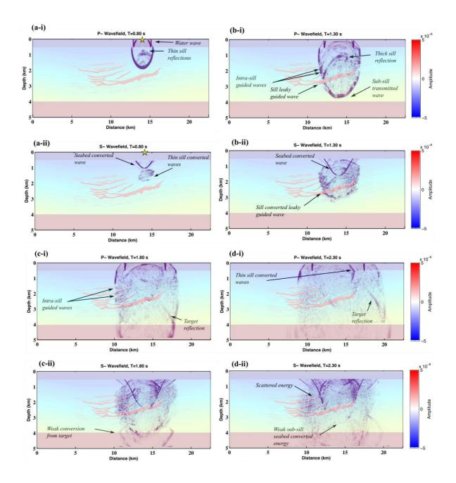
Figure 3: Snapshots of seismic wave propagation for 'Shot 2' (yellow star) after 0.80 (a), 1.30 (b), 1.80 (c) and 2.30 (d) seconds for the P- (i) and S- (ii) wavefield.
