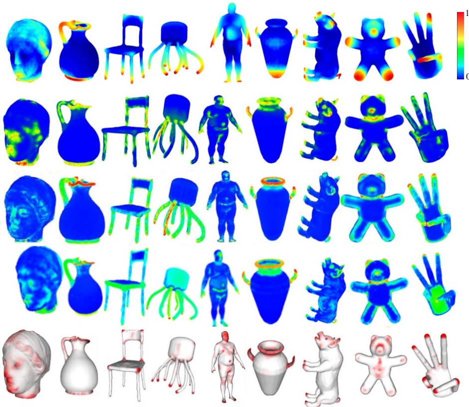
Fig. 5. Comparisons with point-based algorithms. Each row represents the saliency visualization of our algorithm, the algorithm by Ding et al. [14], the algorithm by Guo et al. [13], the algorithm by Tasse et al. [12], and the ground truth provided by Chen et al. [15], respectively. From left to right, the models shown are egea, kettle, chair, octopus, human, vase, pig, teddy, and hand. In each model, the areas that are closer to red indicate higher saliency.
