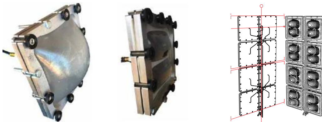
Figure 5: Test jig assembly with composite hard plastic / shape memory polymer sample.
