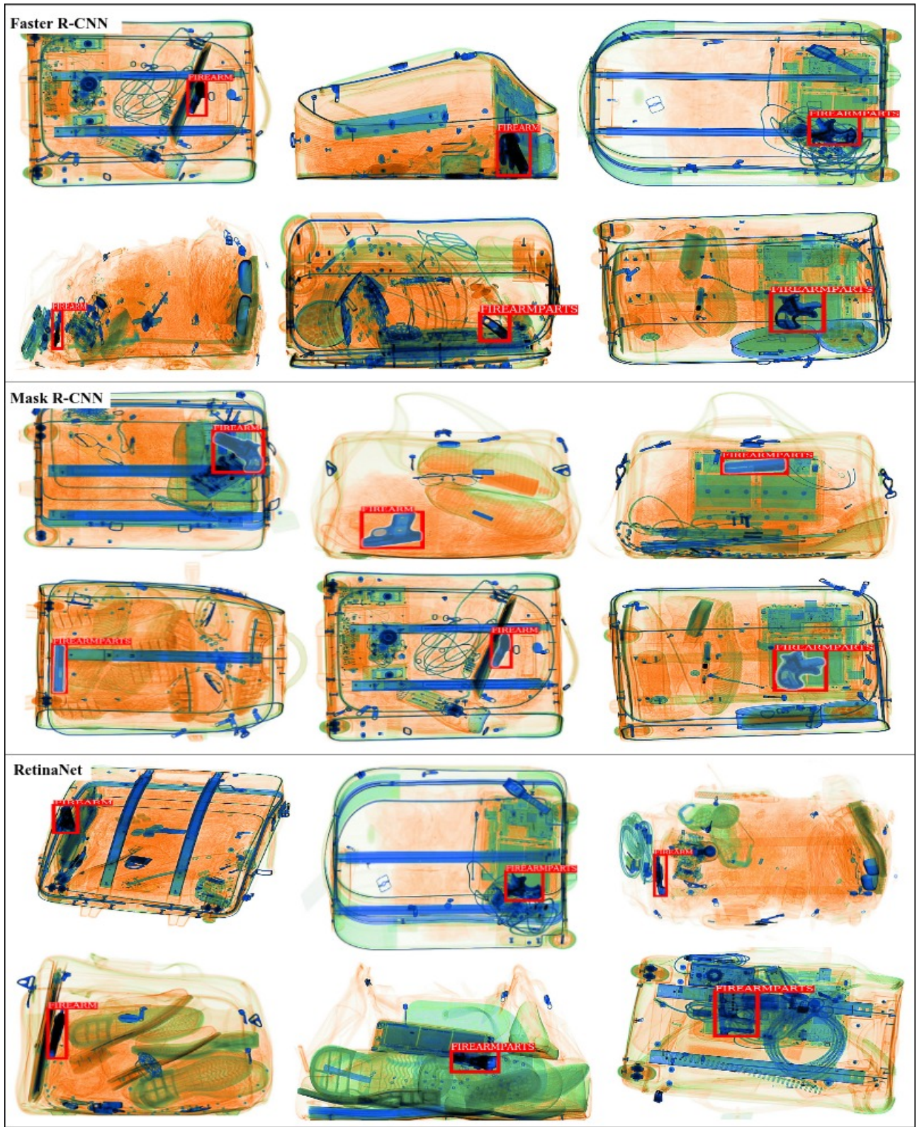
Fig. 3. Threat item (Firearm, Firearm Components) detection in X-ray security imagery by using CNN architecture such as Faster R-CNN [11], Mask R-CNN [12] and RetinaNet [13] on Dbf2 .
