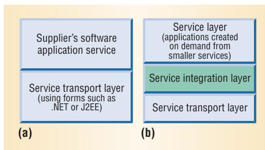
**Figure 1. Service models. (a) The current supply-led service model provides only a predetermined range of services from a remote server. (b) The proposed demand-led service model has a service integration layer inserted above the transport layer.**
