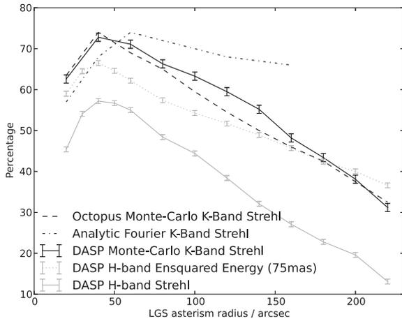
**Figure 2.** On-axis *K*-band Strehl ratio (black lines) as a function of the LGS asterism radius. The black solid curve presents the DASP results that we have obtained, the dashed curve is from the ESO OCTOPUS Monte Carlo simulation and the dot-dashed is from an analytic Fourier code. For comparison with the remainder of this paper, *H*-band results are also shown in grey, with dotted grey being ensquared energy within 75 mas and solid grey being the Strehl ratio.
