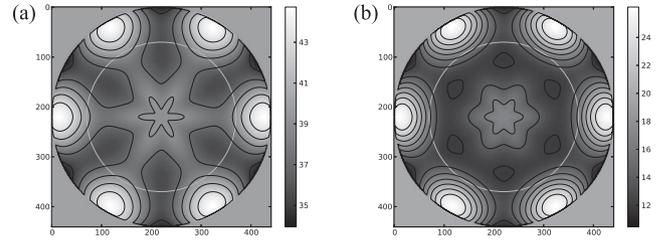
**Figure 4.** (a) *H*-band MOAO performance (ensquared energy in  $75 \times 75$  mas) over the 440 arcsec technical field of view of an EAGLE-like instrument, with an LGS asterism diameter of 440 arcsec. The centred grey circle represents a 5 arcmin field, and contours are spaced by 2 per cent, starting at 35 per cent ensquared *H*-band energy. (b) As for (a), showing the Strehl ratio over the field.
