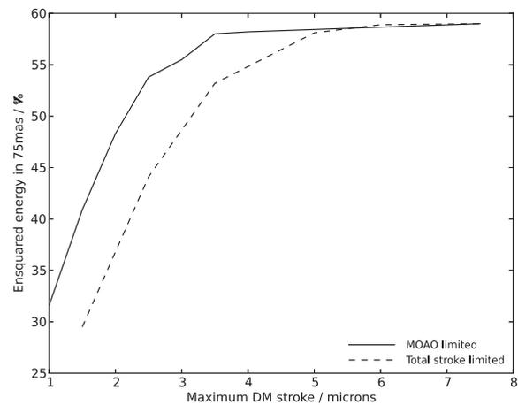
**Figure 6.** AO performance as a function of the maximum MOAO DM stroke (solid) for an LGS asterism with 20 arcsec radius. Also shown (dashed) is performance when total stroke is limited (i.e. assuming that the GLAO correction is not present).
