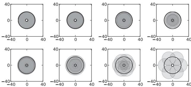
**Figure 3.** LGS overlap at different atmospheric heights for an asterism radius of 40 arcsec (top row) and an asterism radius of 220 arcsec (bottom row). The LGS beacon is focused at 90 km, and overlap at 2.25, 4.5, 9 and 18 km is shown. The scale is in metres.
