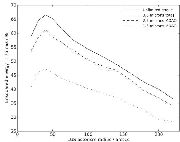
**Figure 7.** AO performance as a function of the LGS asterism radius, for an MOAO DM with unlimited stroke (solid), a maximum stroke of 2.5  $\mu\text{m}$  (dashed) and a maximum stroke of 1.5  $\mu\text{m}$  (dotted).
