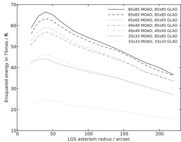
**Figure 5.** AO performance as a function of the LGS asterism radius for the different DM actuator counts given in the legend. A ground-layer (GLAO) correction followed by an MOAO correction (with no ground-layer component) is performed. Stroke is unlimited for both DMs. It should be noted that cases with equal order for both GLAO and MOAO DMs are identical to a case using only an MOAO DM of the same order that includes ground-layer correction and is not stroke limited.
