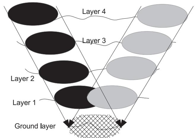
**Figure 1.** The separation of GLAO and MOAO DM correction. The GLAO DM (hatched) is used to perform a global ground-layer correction, while the MOAO DMs (one performing correction of light grey areas and one performing correction of dark grey areas) only correct higher layers along individual lines of sight and perform no additional ground-layer correction.
