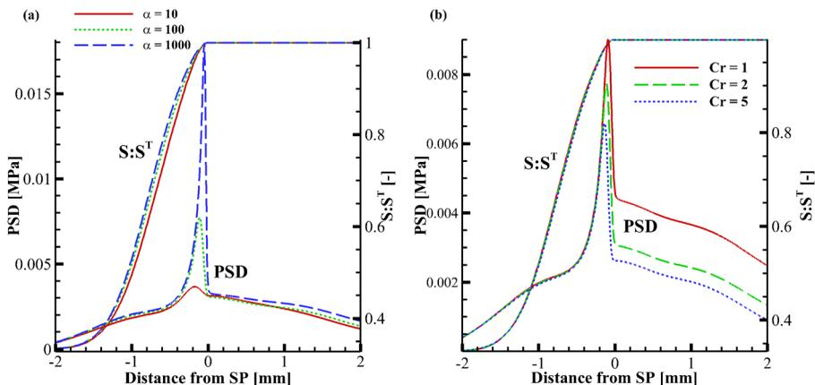
**FIG. 5.** PSD and  $S : S^T$  along the SP streamline as a function of distance from the SP showing variations in (a)  $\alpha$  and (b)  $C_R$ . Negative distance from the SP corresponds to the inlet channel and positive distance the outlet channel.
