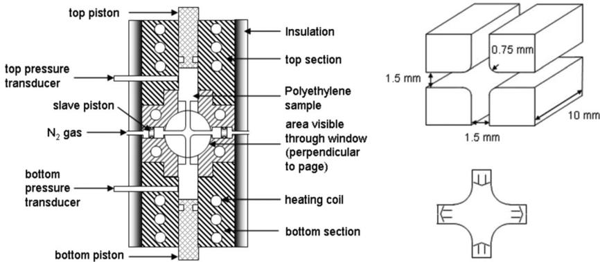
FIG. 1. (a) Schematic outlining the Cambridge MPR core and (b) the dimensions and flow direction for the cross-slot geometry insert as used in the midsection of the MPR. The associated flow directions are indicated by arrows.
