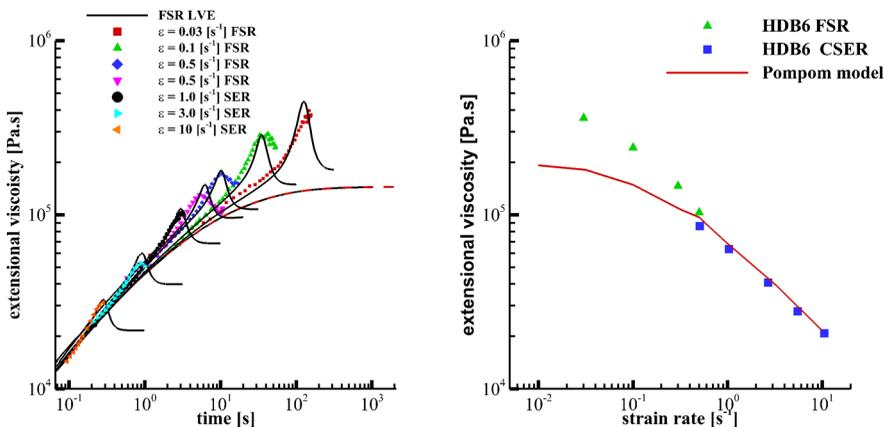
FIG. 9. The transient (a) and steady-state (b) data for HDB6 are plotted along side the OPP model fitted to the data (lines). For the transient fit, the slower strain rates were measured by the FSR and the higher rates by the SER. The steady-state data came from the FSR and the CSER.
