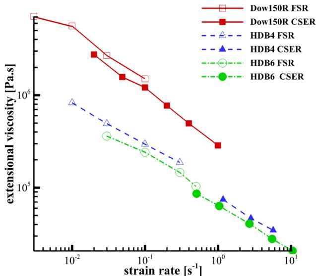
**FIG. 6.** A comparison of the steady-state extensional viscosity measurements from the FSR and the CSER for three polyethylene samples detailed in Table I. The open symbols show the FSR results and the closed symbols show the CSER data.
