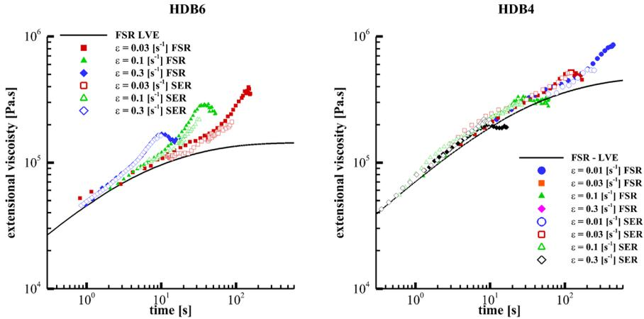
**FIG. 7.** A comparison between the transient extensional stress response as measured by the FSR (closed) and the SER (open) for HDB6 (left) and HDB4 (right). The figure shows a good agreement of the initial stress growth, until sample rupture limits the SER to Hencky strains of around 4.
