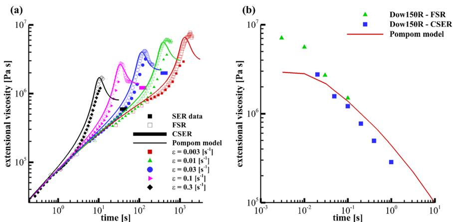
**FIG. 8.** (a) A plot comparing extensional data and OPP theory for Dow150R. Strain rates range from 0.003 to  $0.3 \text{ s}^{-1}$ . The closed symbols show the SER data and the open symbols data from the FSR achieving higher Hencky strains than the SER. The lines show the theoretical prediction from the OPP model. (b) The steady-state extensional viscosity values from the FSR and the CSER are compared to the prediction of the Pompon model fitted to the data.
