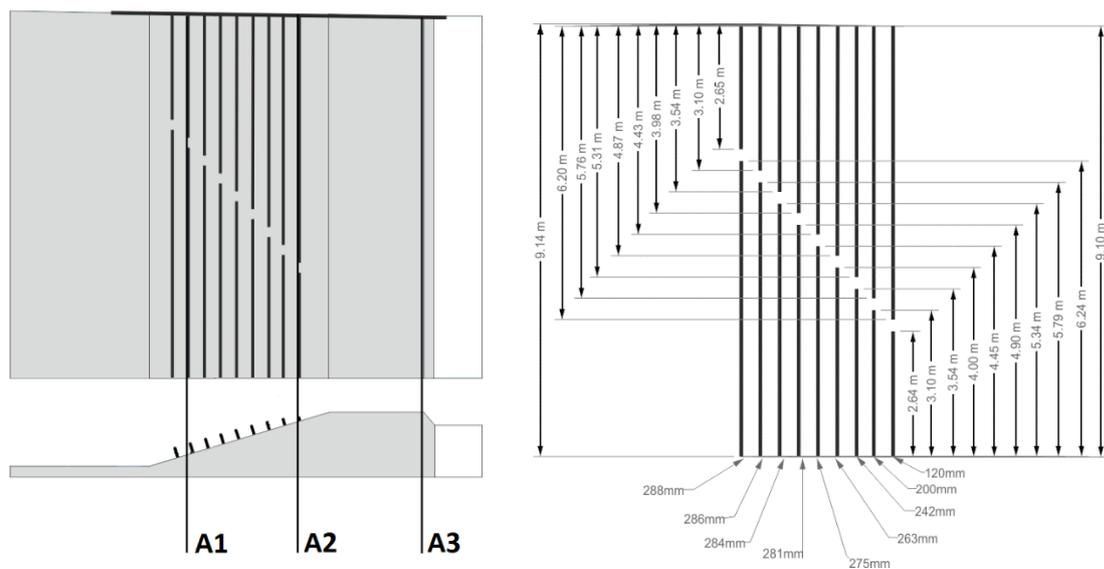
**Fig. 2. Left: Plan view of the LCB arrangement on the Hogsmill weir apron with positions of antenna placement. Right: Schematic of the height and length of each baffle placed on the Hogsmill weir apron. The width of the notch in each baffle is 250 mm. The space between each baffle is 400 mm. River flow for both left and right panels is from right to left.**
