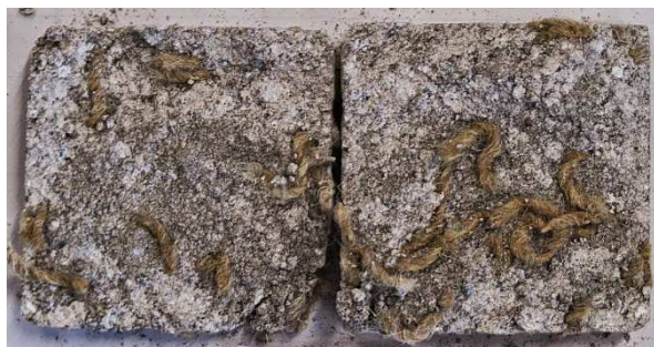
Fig. 5: Photograph showing the top (L) and bottom (R) halves of the fracture plane of sample ID W1C4-1.
