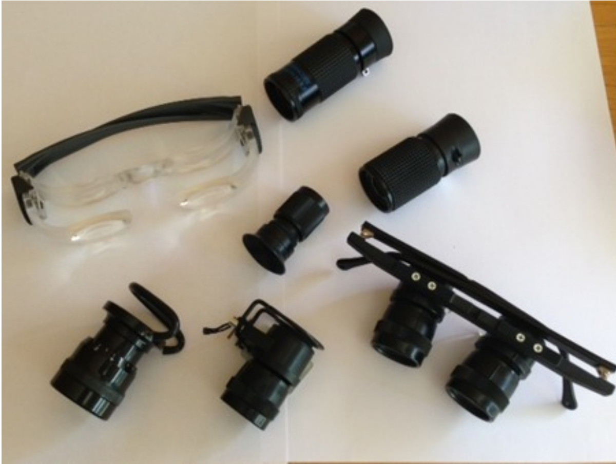
Figure 2. A selection of currently available telescope Low Vision Aids, showing devices cfor a range of distances. Reproduced from ref 10
