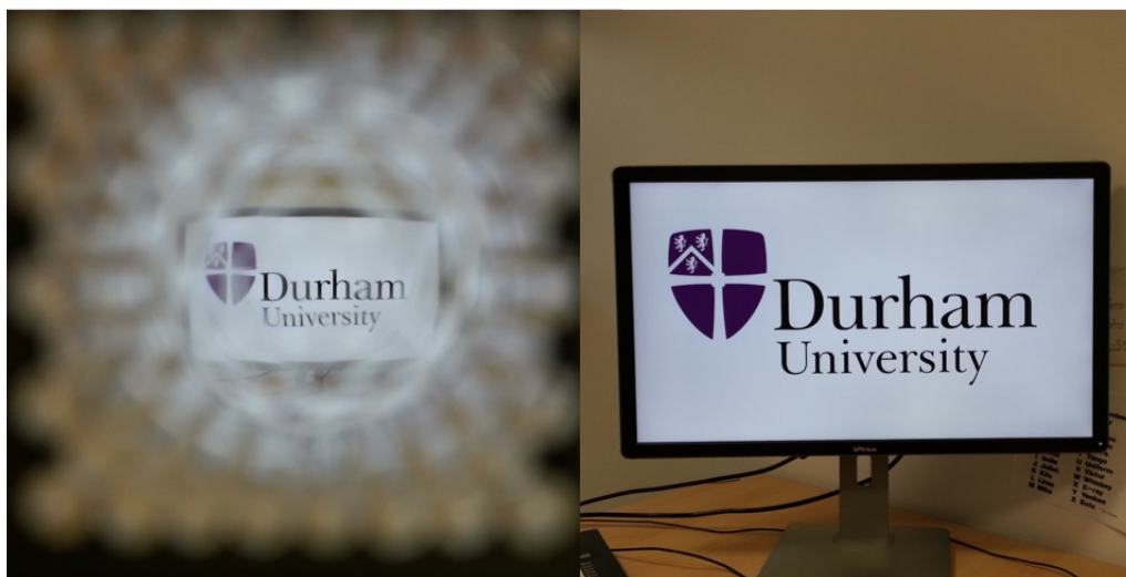
Figure 6. The phase 2 device, shown here in demagnifying orientation. A clear "tunnel" of unwanted light can be seen around the core image.
