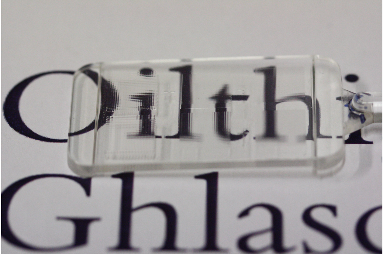
Figure 3. The phase one device, referred to as a "paddle". Visible are the 6 different sub-arrays we designed for phase 1. Only 3 of the 6 had the rear lenslet machined as it was already apparent from the larger lenslets that the aperture widths were too small. As such the diffraction effects would have been so high as to introduce a large diffractive blur.
