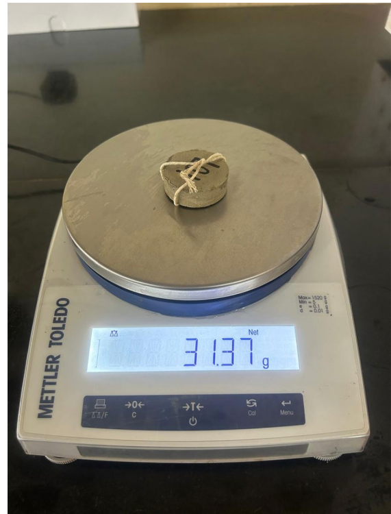
Fig. 11 A typical view showing recording the mass of dry soil pat coated with hydrophobic compound along with cradle after being removing from submersion
