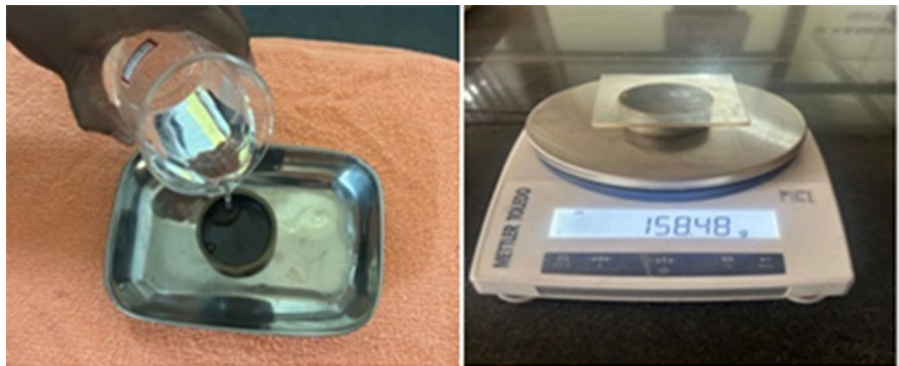
Fig. 3 View showing recording the mass of shrinkage dish filled with water along with glass plate
