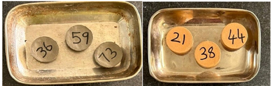
Fig. 7 A typical view showing the shrinkage pats coated with hydrophobic glue
