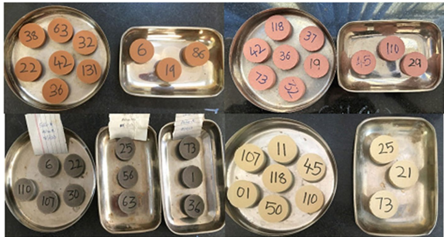
Fig. 4 A typical view showing dry shrinkage pats of few soils used in the study with numbering for identification
