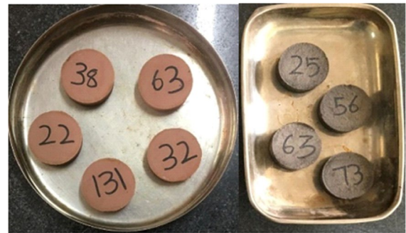
Fig. 5 A typical view showing the shrinkage pats coated with vaseline
