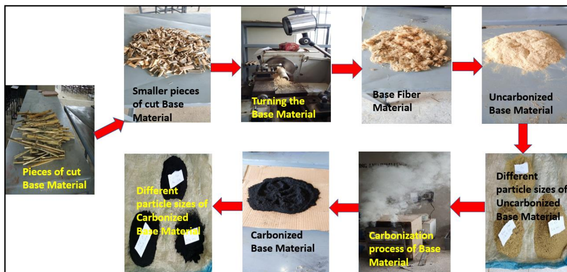
Figure 2. Flow chart of the carbonization process
