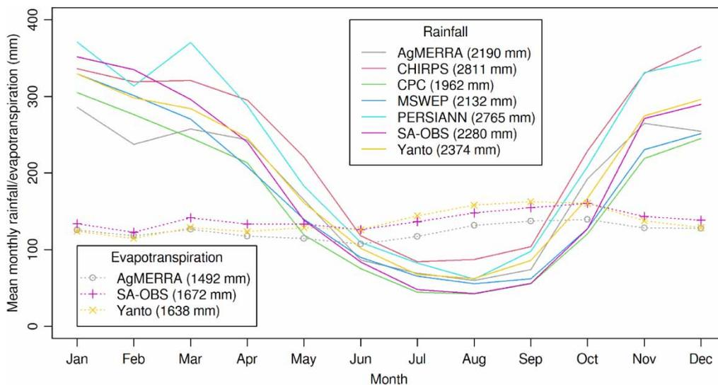
**Figure 2** | Mean monthly precipitation and evapotranspiration in the Citarum basin during 1985–2010. Bracketed values in legends indicate the mean annual total during 1985–2010.
