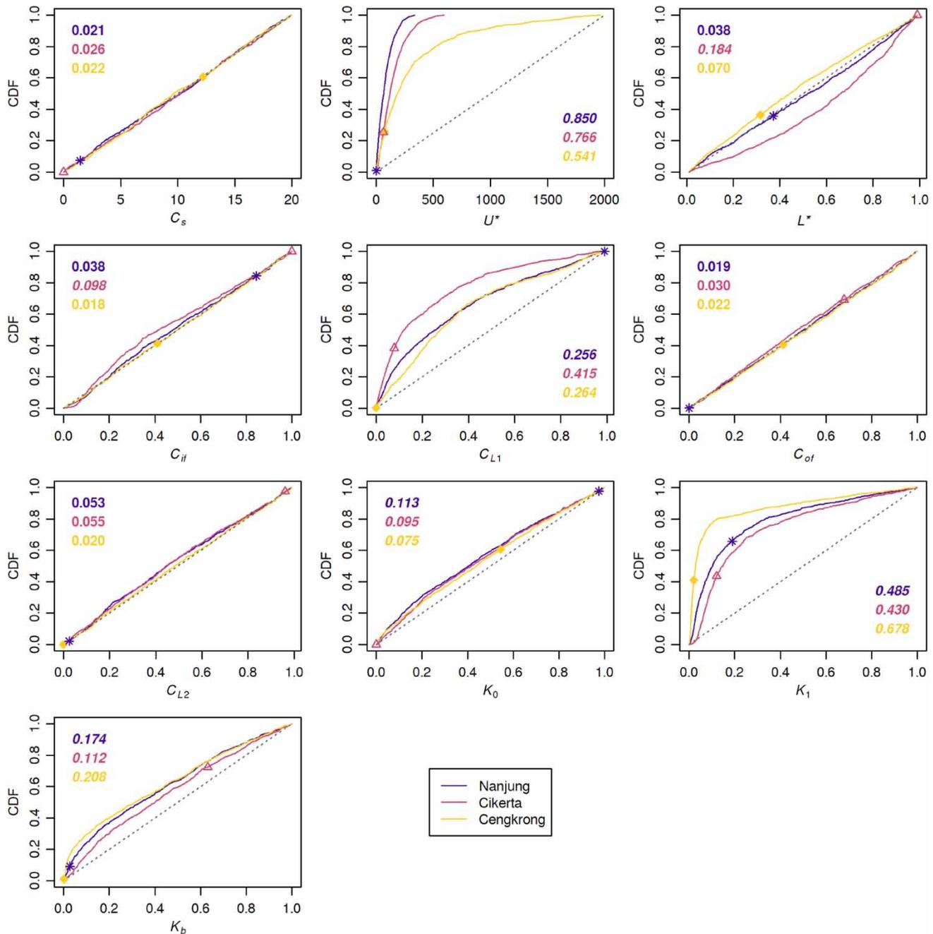
**Figure 8** | Cumulative distributions for NAM parameters, corresponding to 100,000 nominally uniform samples for each parameter (dotted grey lines), the 1,000 samples giving the highest  $KGE'$  scores compared to gauged flow data for each catchment (coloured lines), and the Stage 1 optimized values for each parameter (coloured symbols).
