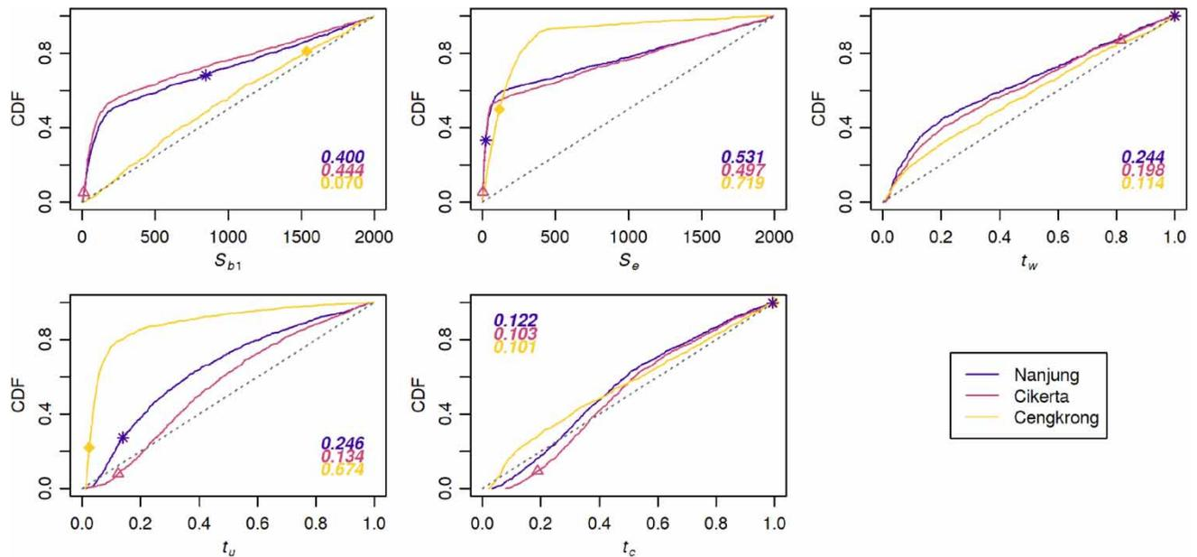
**Figure 7** | Cumulative distributions for MOPEX-1 parameters, corresponding to 100,000 nominally uniform samples for each parameter (dotted grey lines), the 1,000 samples giving the highest  $KGE'$  scores compared to gauged flow data for each catchment (coloured lines), and the Stage 1 optimized values for each parameter (coloured symbols).
