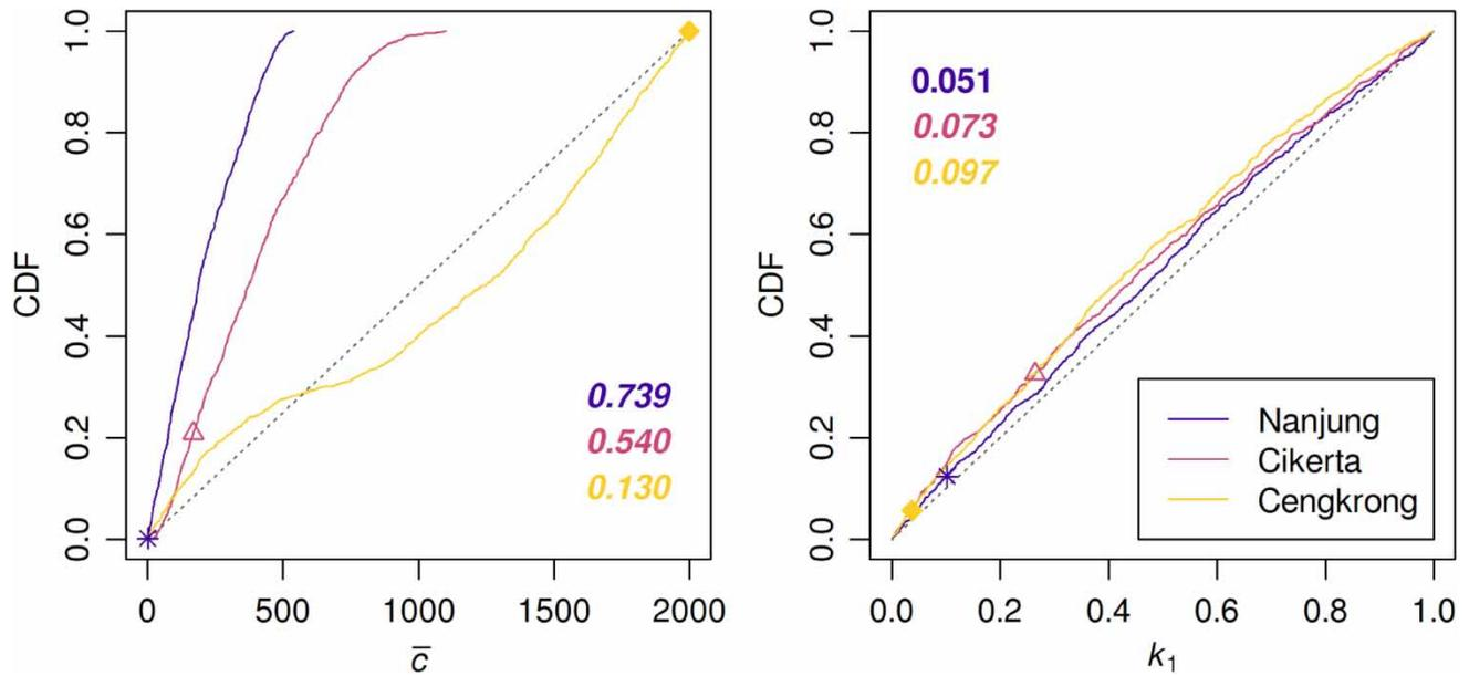
**Figure 9** | Cumulative distributions for two-parameter PDM parameters, corresponding to 100,000 nominally uniform samples for each parameter (dotted grey lines), the 1,000 samples giving the highest  $KGE'$  scores compared to gauged flow data for each catchment (coloured lines), and the Stage 1 optimized values for each parameter (coloured symbols).
