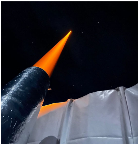
Figure 1. A photo of the 70 W LGS at the Wendelstein LGS unit in La Palma, Canary Islands, Spain.
