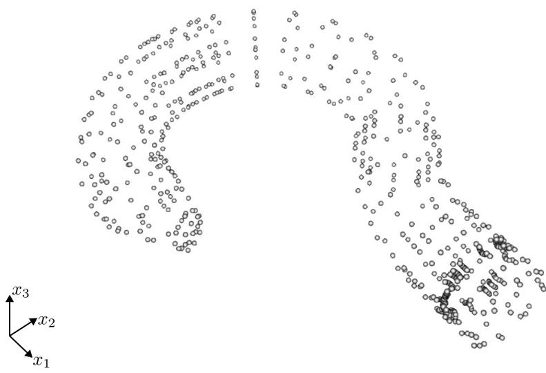
Figure 29: Collocation points position for the XIGABEM model of hook with crack.
