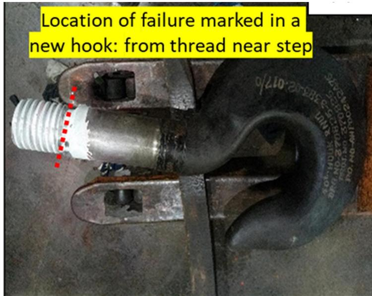
Figure 27: Fatigue crack location in crane hook experiment [71].
