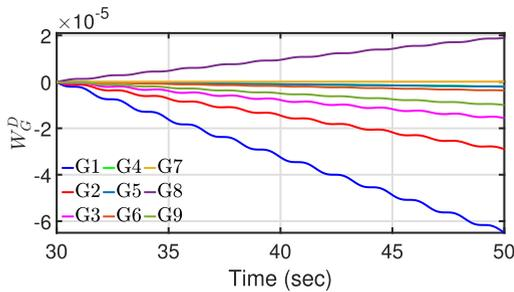
**FIGURE 4.** IEs of generators for forced oscillation frequency  $f = 0.6$  Hz (zoom in G1-G9) in the 10-machine 39-bus system.
