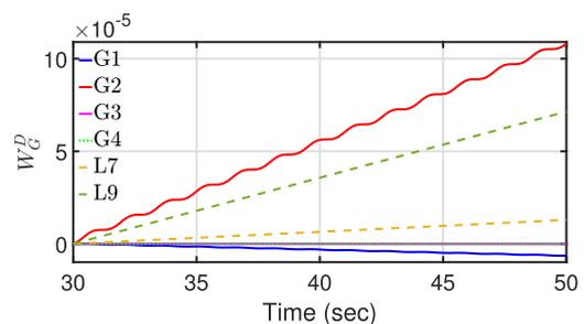
FIGURE 3. IEs of generators for forced oscillation frequency *f* = 0.66 Hz in the 2-area 4-machine system.
