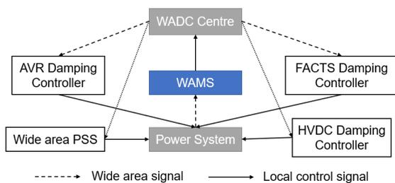
FIGURE 2. Basic framework of wide-area damping control [13].
