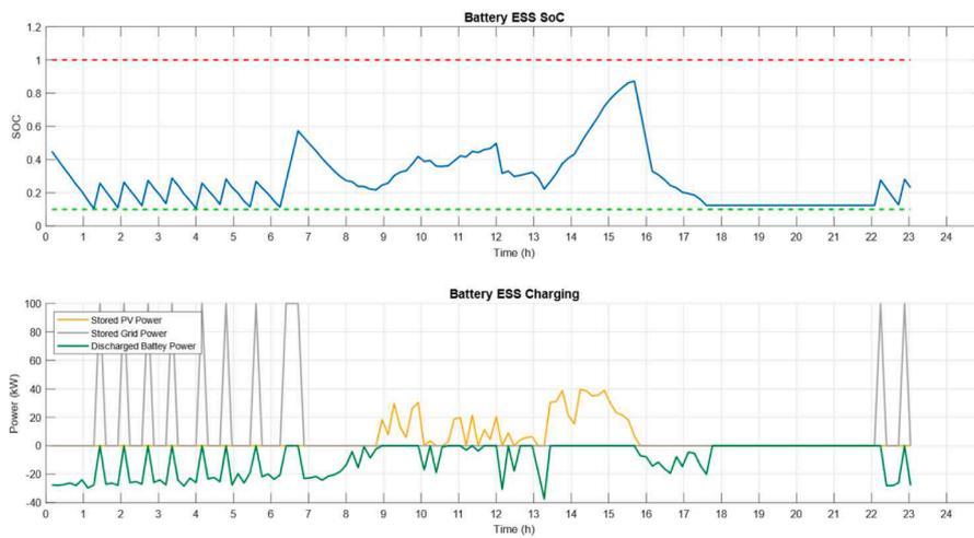
Fig. 25. BESS charging, discharging and SOC profiles for scenario 1.
