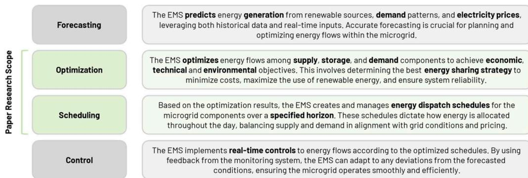
Fig. 3. EMS core functions and the paper's research scope.
