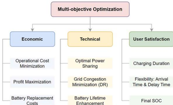
Fig. 9. Microgrid multi-objective optimization targets.
