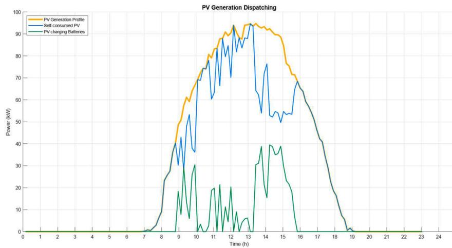
Fig. 24. PV generation dispatching for scenario 1.
