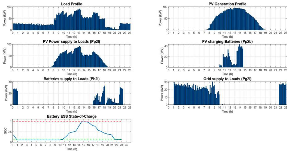
Fig. 18. Power dispatching results for scenario 0.
