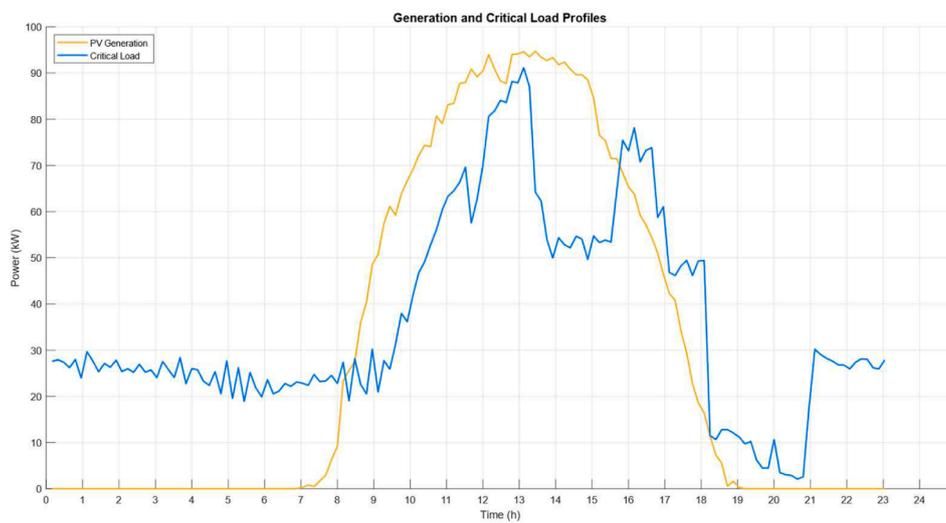
Fig. 16. Microgrid's generation and consumption profiles of a typical day.
