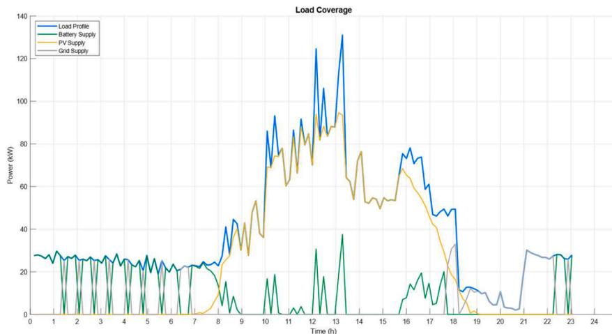
Fig. 23. Load coverage for scenario 1.
