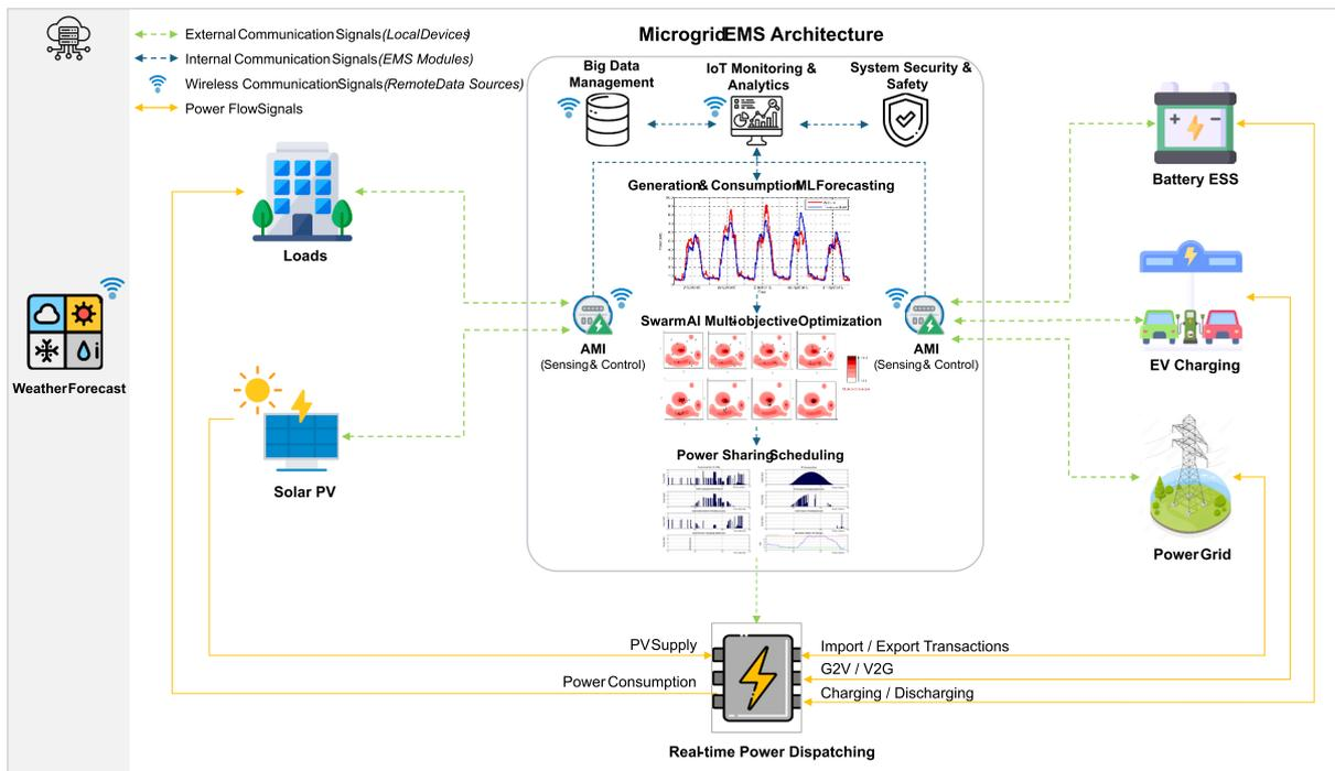
Fig. 4. Proposed microgrid EMS architecture.
