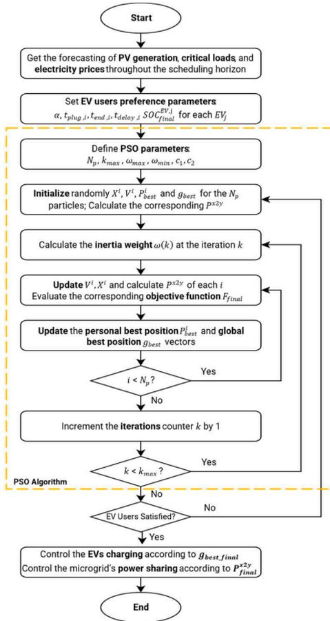
Fig. 14. Proposed microgrid EMS's algorithm flowchart.
