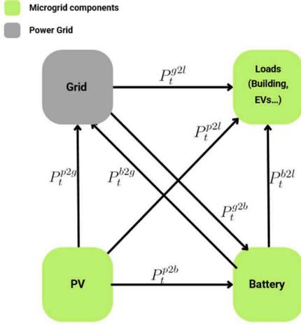
Fig. 5. Power exchange among the microgrid components.
