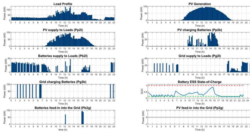
Fig. 21. Power dispatching results for scenario 1.
