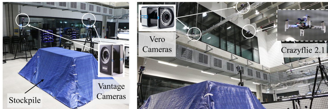
Figure 4. Views of the netted drone flight test enclosure. Highlighted are the advanced VICON motion tracking system components. The inset image also showcases the Crazyflie 2.1 drone in action while above the blue stockpile.
