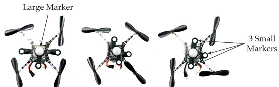
Figure 5. Crazyflie 2.1 drones equipped with four, one large and three smaller, markers for accurate tracking during the experiments.
