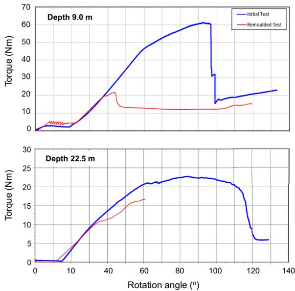
**Fig. 2 | Evidence of microstructure in vane shear test results.** Results of the vane shear tests VT-16-11 (Depth 9.0 m) and VT-16-12 (Depth 22.5 m) on the Brumadinho tailings (with permission, after Robertson et al.<sup>3</sup>).
