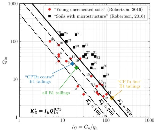
**Fig. 1 | Evidence of microstructure in CPT results.**  $Q_{tn}$  vs  $I_G$  chart to identify soils with microstructure (after Robertson<sup>2</sup>).
