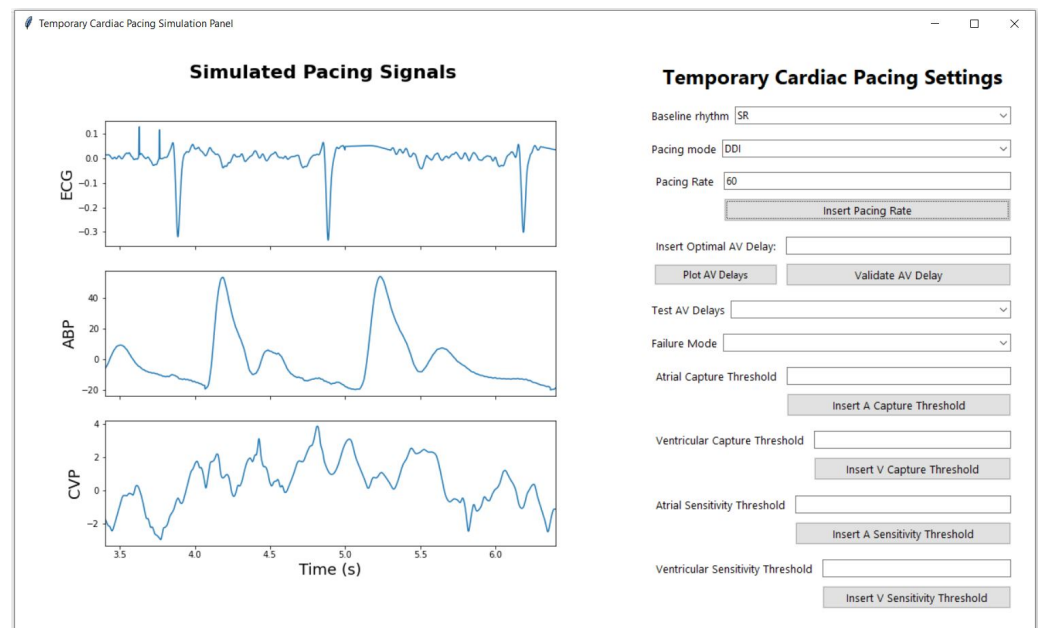
Figure 16. Example of the signal displayed when the user selects the baseline signal, in this case, SR, and chooses the DDI pacing mode with a pacing rate under 70 bpm, causing the intrinsic conduction to show on the signals and the inhibition of the pacing spikes in both the atria and the ventricles, where intrinsic conduction occurs.
