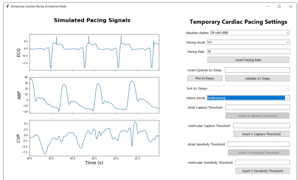
Figure 19. Example of the signal displayed when the user selects the SR with LBBB baseline rhythm and chooses the VVI pacing mode with a pacing rate of 80 bpm, while also selecting “undersensing” from the failure mode dropdown menu. In undersensing failure mode, the TCPS shows pacing spikes erroneously superimposed on the T-waves. These inappropriate spikes occur due to the TP’s failure to correctly sense the heart’s intrinsic activity, leading to the delivery of pacing stimuli during the repolarization phase.
