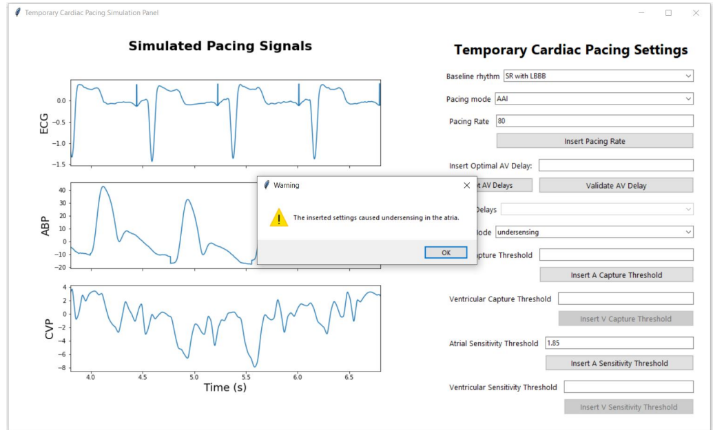
Figure 29. Atrial Sensitivity Threshold Test: This figure depicts the signal output when the user selects LBBB as baseline rhythm and sets the pacing mode to AAI at a rate of 80 bpm. The user inputs a value for the atrial sensitivity threshold and clicks the “Insert A Sensitivity Threshold” button. The TCPS system compares this input against a predefined maximal atrial sensitivity threshold. In this case, the entered threshold fails to capture the atria, prompting the TCPS to automatically switch the failure mode to undersensing. A warning message is then displayed, informing the user that the selected threshold has caused undersensing in the atria.
