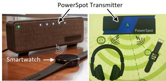
FIGURE 26. Far-field RF wireless charging system for smartwatches [144], [145].
