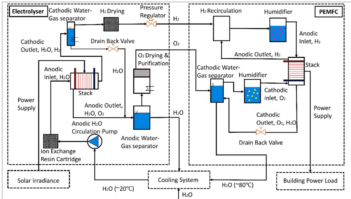
Fig. 2. Schematic diagram of the proposed system.
