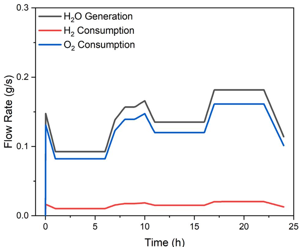
Fig. 8. PEMFC's H<sub>2</sub>O generation, H<sub>2</sub> consumption and O<sub>2</sub> consumption.
