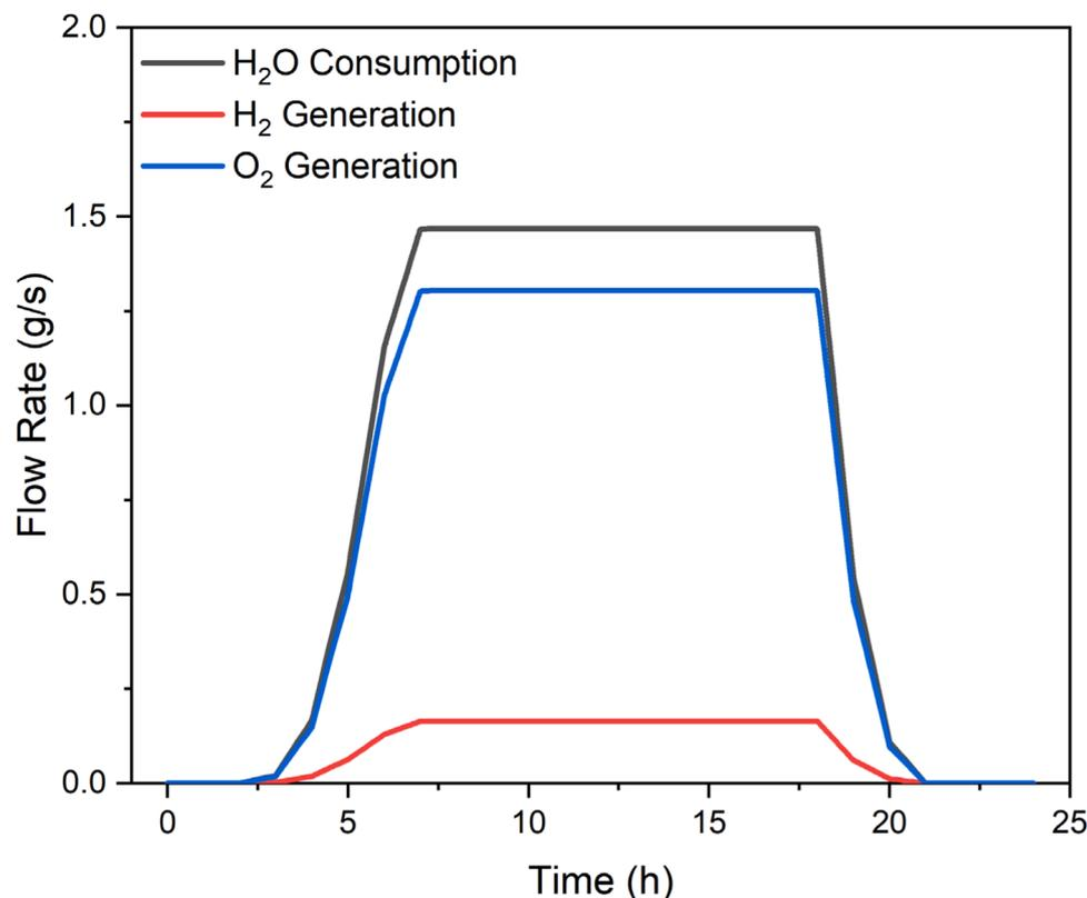
Fig. 7. Electrolyser's  $H_2O$  consumption,  $H_2$  generation, and  $O_2$  generation.
