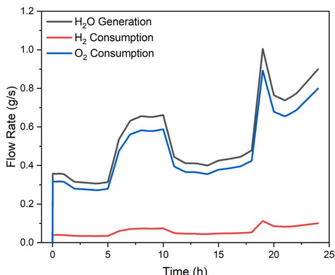
Fig. 11. PEMFC's H<sub>2</sub>O generation, H<sub>2</sub> consumption, and O<sub>2</sub> consumption.
