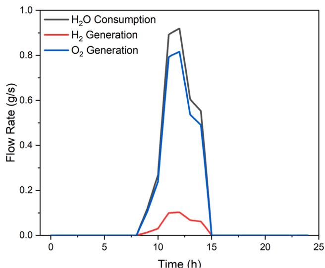
Fig. 10. Electrolyser's H<sub>2</sub>O consumption, H<sub>2</sub> generation, and O<sub>2</sub> generation.
