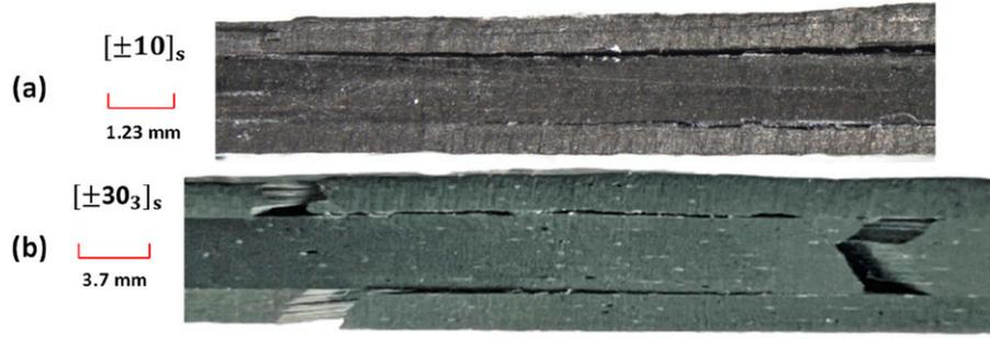
**Figure 11.** Delamination at the (a) +10/−10 interface of  $[\pm 10]_s$  and (b) +30/−30 interface of  $[\pm 30]_s$  monolithic angle-ply laminates.
