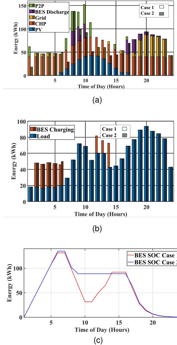
Fig. 2. Energy schedule of (a) sources; (b) load; and (c) BES.
