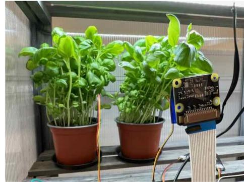
**Figure 2: A mini-greenhouse with basil plants and sensors.**
