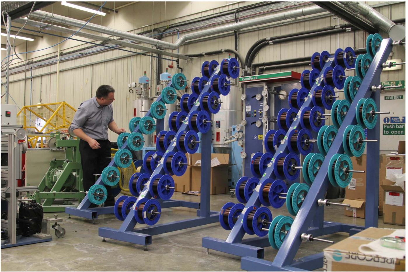
Figure 22. Manufacturing bundles of science fibers inside Miniflex conduit in a collaboration between Durham University and PCC Broadband Fiber Ltd.
