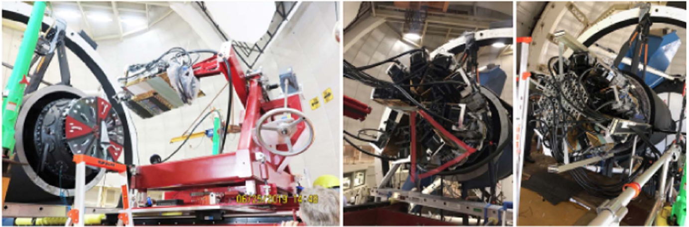
Figure 40. The panel on the left shows the first petal loaded onto the sled prior to insertion. The sled ensures that the petal is well aligned before it is inserted in order to reduce the risk of damage to the fiber positioners. The panel in the middle shows the back of the focal plane with 8/10 petals installed. The panel on the right shows the cable management structure that ensured that the bend radius of the cables would not be exceeded and that each cable could be moved without affecting any other cable.
