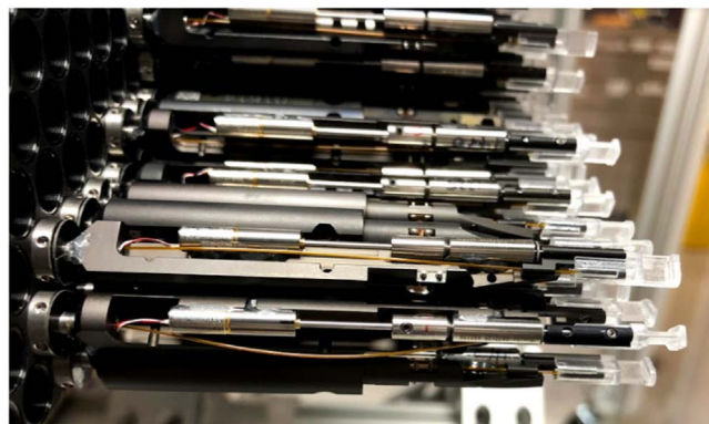
Figure 46. A fiber can be seen bowing out of the edge of the positioner. This is due to the ferrule being fixed into the ferrule arm and the Hytrel tubing adding electrostatic stickiness on the fiber and causing it to be pushed, inchworm style, into the positioner. This issue was remedied by shortening the amount of Hytrel tubing on the fiber.
