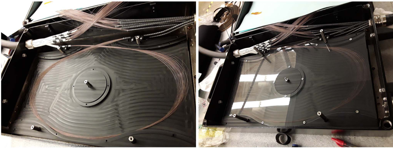
Figure 24. A spectrograph spool box tray populated with bare looped fiber. A clear Perspex lid is installed, which allows the fiber technician to ensure that all fibers are able to move freely inside the cassette before building the next bundle.
