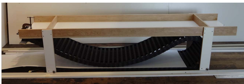
Figure 13. Panel (a) shows the route of the fiber cables around the decl. axis. The cables route around this axis in the e-chain, and to test the load that this would place on the telescope bearing, we loaded 10 short lengths of cable into a section of the e-chain and measured the force required to roll and unroll the bundle. Panel (b) shows the lab setup. A force gauge was attached to the top tray and the force as the cable was rolled and unrolled was measured. The tests were performed at speeds much faster than the slew rate of the telescope. The results are shown in panel (c) and the results reassured us that the movement of the telescope would not be impeded with this routing design.
