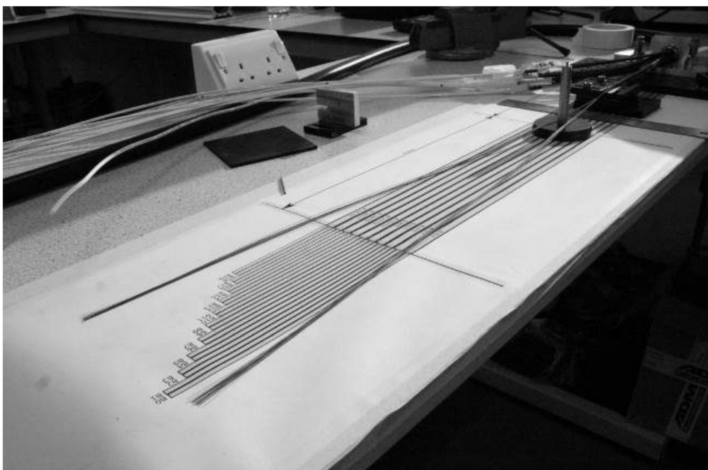
Figure 32. A to-scale paper template is used to set the appropriate lengths for the bare and PTFE-clad fiber bundles. Each bundle had a unique length to conform to the “race track” slots of the slit assembly.
