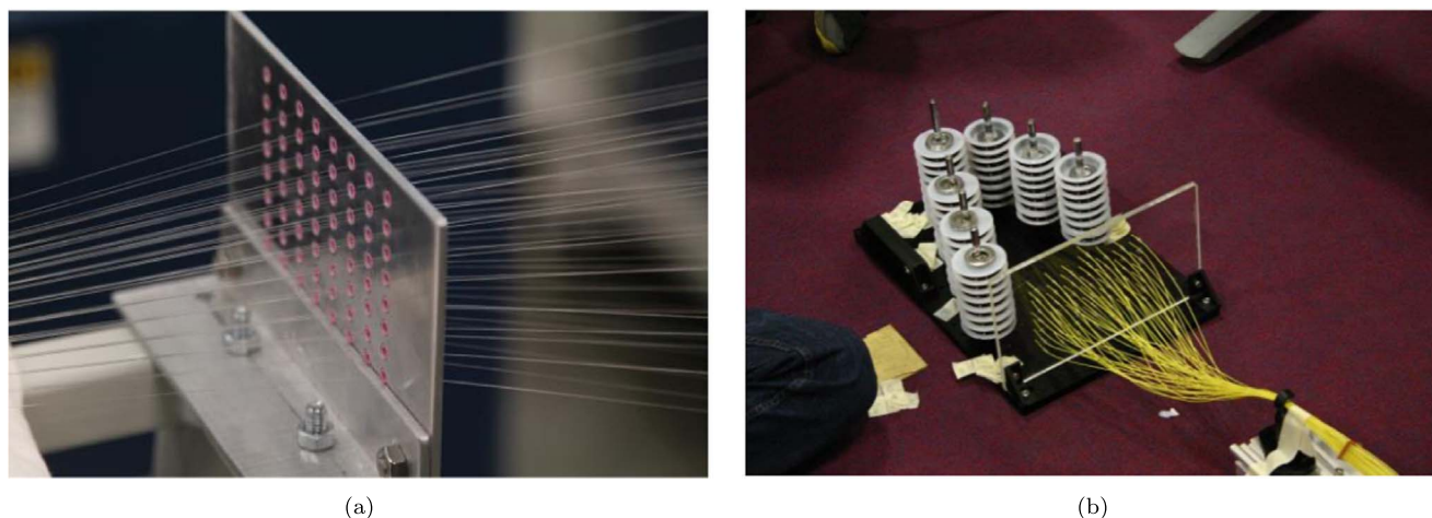
Figure 14. Panel (a)—A bare fiber bundle inserted into a Miniflex conduit having passed through the mandrel with ceramic eyelets. Panel (b)—Experimental 50 m fiber cable draw inserted into Miniflex conduit with individual fiber reels and a deterministic fiber feed using a mandrel of low-friction, low-static PTFE tubes plus a deionizer.
