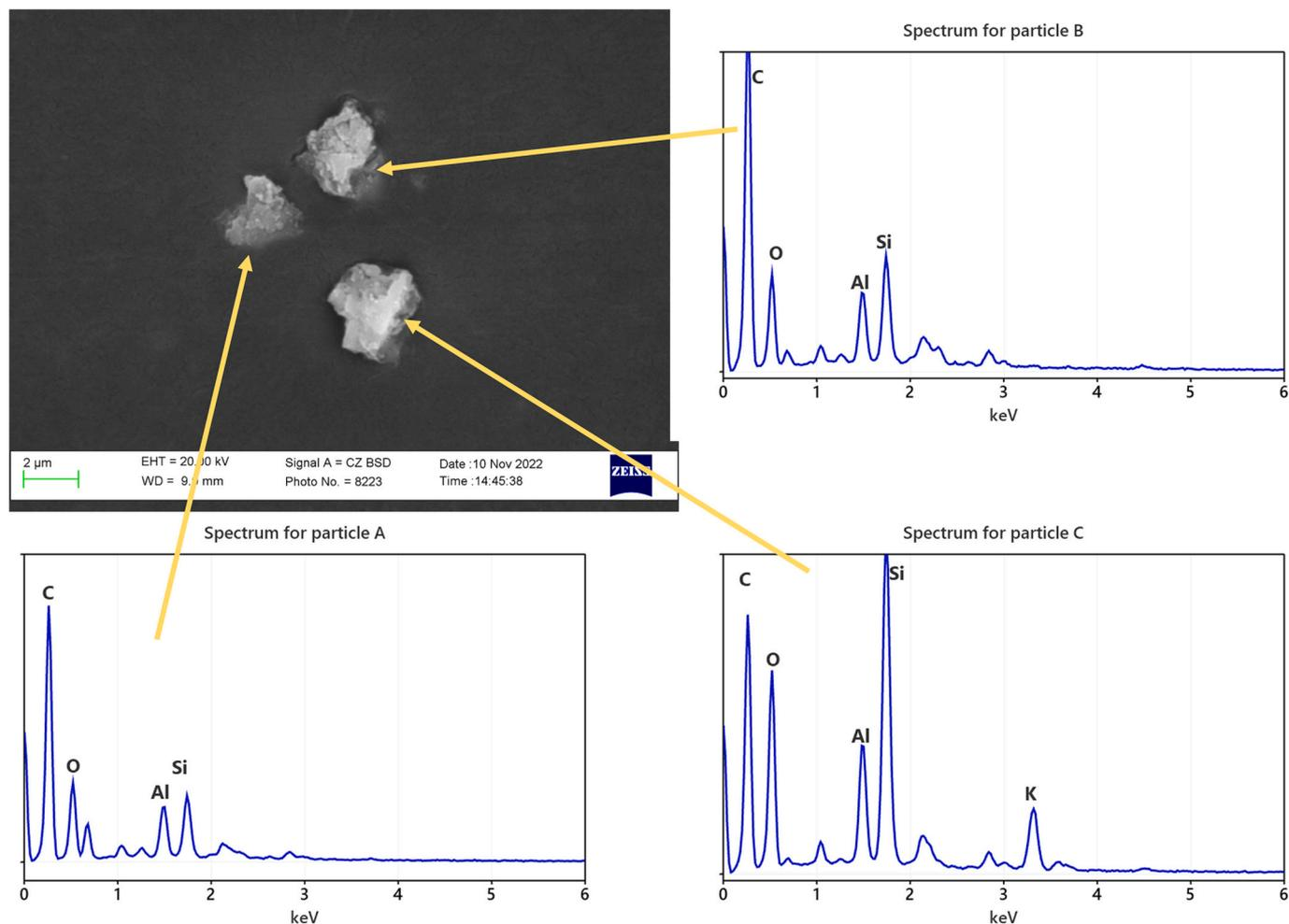
Fig. 2. Example of SEM backscattered electron image of 3 PM<sub>10</sub> particles and corresponding energy dispersive x-ray (EDX) microanalysis spectra.
