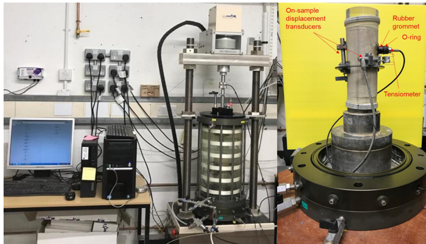
Fig. 1. Photograph of GDS triaxial testing apparatus and on-sample instrumentations
