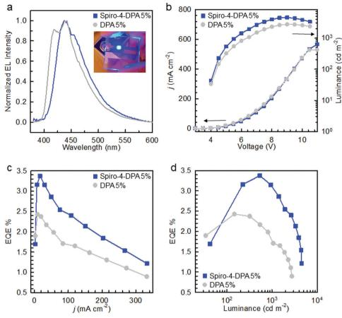
Figure 3. a) Electroluminescence (EL) spectra of the spiro-4-DPA and DPA (5 vol% in CBP) OLED devices at 5.5 V applied voltage. b) Current density and luminance of the investigated devices as a function of the applied voltage. OLED external quantum efficiency (EQE) as a function of c) the injected current density and d) OLED luminance.
