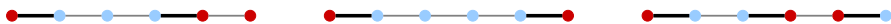
Fig. 1 The graph P_6 with a matching cut that is not contained in a disconnected perfect matching (left), a matching cut that is properly contained in a disconnected perfect matching (middle) and a perfect matching cut (right). In each figure, thick edges denote matching cut edges
