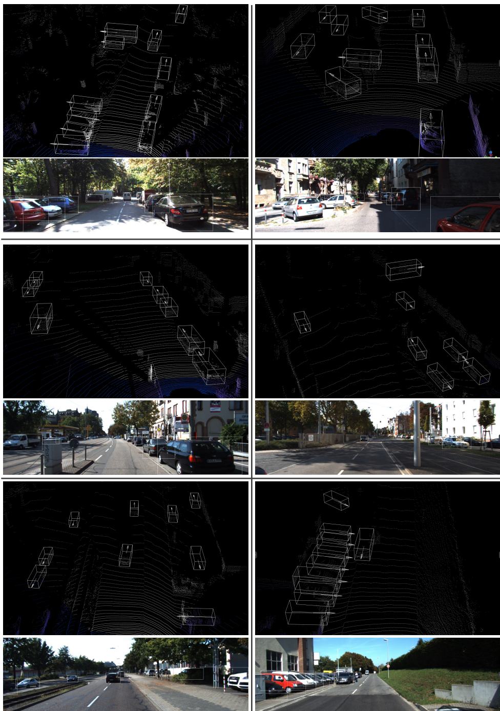
Figure D1: Qualitative results of 3D object detection with our TraIL-Det on KITTI dataset. The predicted 3D bounding box is labeled in the LiDAR point cloud, while its corresponding 2D bounding box is labeled in the RGB image. In the point cloud, white points represent points within the camera field of view (FOV), and purple points indicate points outside the camera FOV. Best viewed in color.
