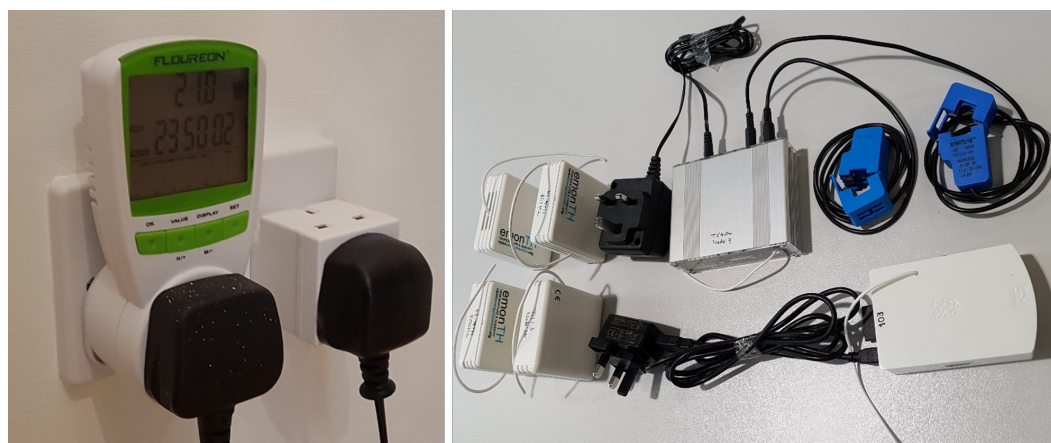
Figure 3. (Left panel): power monitor used to characterize household appliances. (Right panel): AC sensor, monitoring transmitters, and temperature sensors deployed in the case study building.
