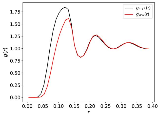
Fig. 5 Radial distribution function between the oppositely charged salt beads and water beads.
