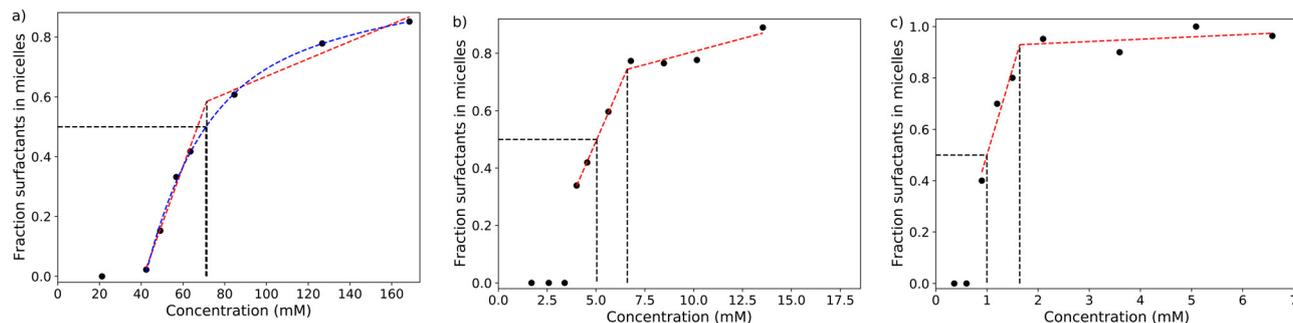
Fig. 6 The fraction of surfactant molecules existing in micelles for S8S (a), S12S (b) and S16S (c). Red linear fits are shown for the purpose of calculating the CMC using method C (as described in the main text). The CMC as determined using method A is also shown, and to identify the point at which  $C_F = C_T/2$ , a blue line of best fit is shown for the S8S surfactant. Calculated CMC values are highlighted by vertical black lines.
