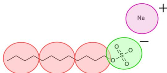
**Fig. 1** Coarse-graining of an SDS molecule such that one tail bead (T) represents four carbon atoms and the head group is represented by a single negatively charged bead (H). The counterion is represented as a partially hydrated positively charged bead (I).
