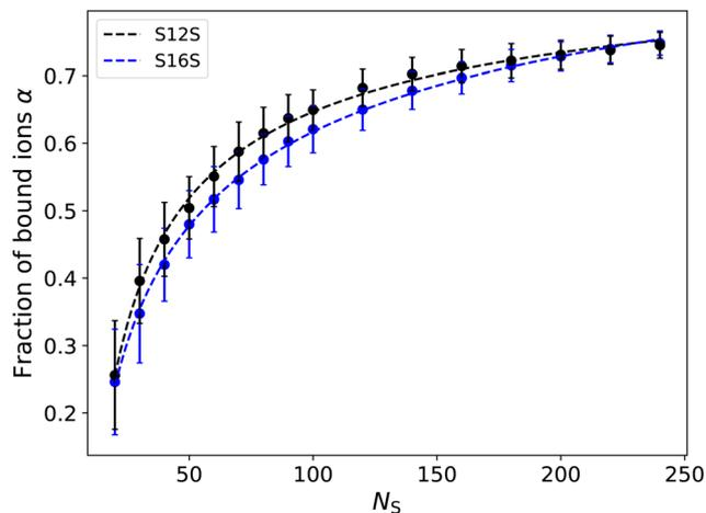
Fig. 13 Fraction of counter-ions bound to the micelle as a fraction of the aggregate size. Bound ions are classed as being those which are within a distance  $r < R_{\text{Ions}} = 0.9$  of a head group. Vertical bars represent the standard deviation over the measurement period (note that standard errors are around the size of the points).
