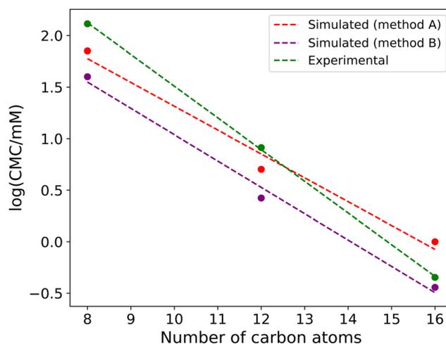
Fig. 7 CMC of alkyl sulfate surfactants as a function of tail length, where simulated results are compared with experimental data obtained from Aniansson *et al.*,<sup>16</sup> who calculate the CMC using conductivity measurements.
