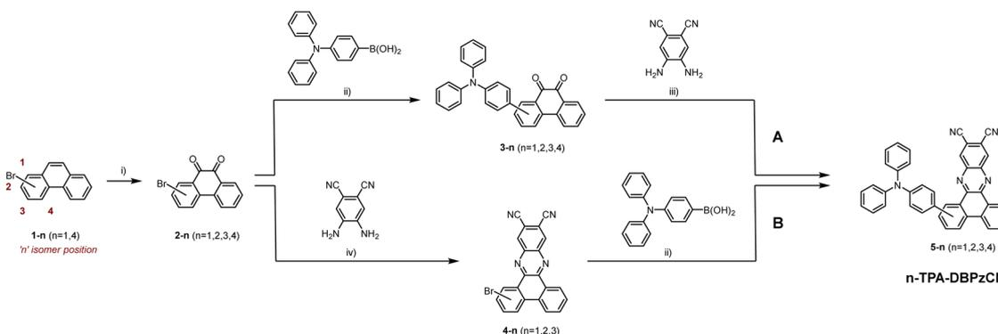
Scheme 1 Synthesis protocol for **1-TPA-DBPzCN**, **2-TPA-DBPzCN**, **3-TPA-DBPzCN**, and **4-TPA-DBPzCN**: (i)  $\text{CrO}_3$ , glacial acetic acid, reflux, 2 h; (ii)  $\text{Pd}(\text{PPh}_3)_4$ ,  $\text{Na}_2\text{CO}_3$ , toluene, water, reflux, 24 h; (iii) HCl (37%), EtOH, THF, 40 °C, 24 h; (iv) glacial acetic acid, reflux, 24 h.
