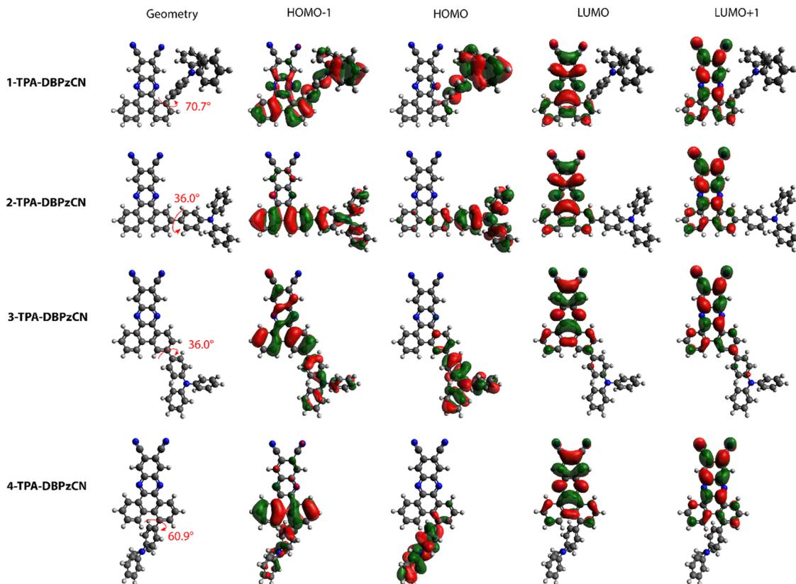
Fig. 3 Optimized molecular geometries and orbital spatial distributions (LUMO+1, LUMO, HOMO, and HOMO–1) for **1-TPA-DBPzCN**, **2-TPA-DBPzCN**, **3-TPA-DBPzCN**, and **4-TPA-DBPzCN**. Values of dihedral angles are given in red. Isocontour values of 0.02 (a.u.) were used for all orbitals.
