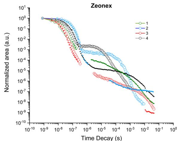
**Fig. 7** Total emission decay (calculated via the integrated area under the emission curve) for **1-TPA-DBPzCN** (green), **2-TPA-DBPzCN** (blue), **3-TPA-DBPzCN** (red), and **4-TPA-DBPzCN** (black) at room temperature (open circles) and 80 K (closed circles). Data points with signal below the noise baseline have been omitted from the figure.
