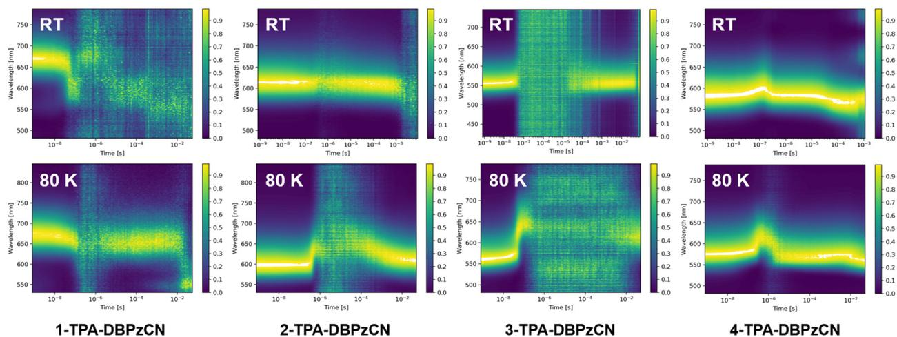
Fig. 6 Normalized time-resolved emission spectra (contour plots) for all isomers in 0.1 w/w% zeonex films ( $\lambda_{exc} = 355$  nm) at room temperature (top row) and 80 K (bottom row).
