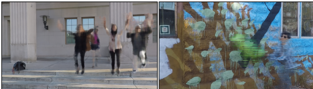
Figure 7: In the absence of global ray sampling point coordinate embedding, the synthesized view displays stripes.
