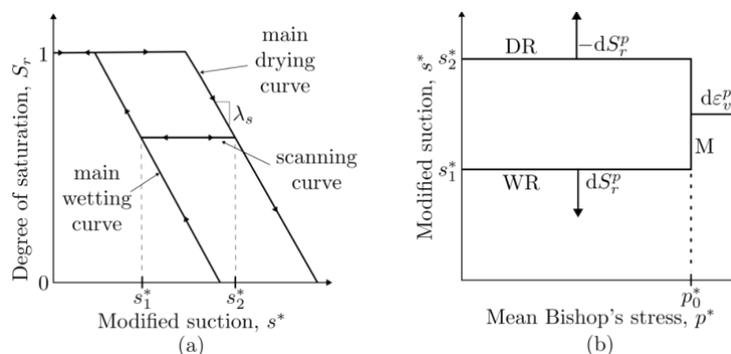
**Figure 1:** The GCM model under isotropic stress conditions: (a) Hysteretic water retention behaviour; (b) Mechanical (M), Drying Retention (DR), and Wetting Retention (WR) yield curves (after [1])
