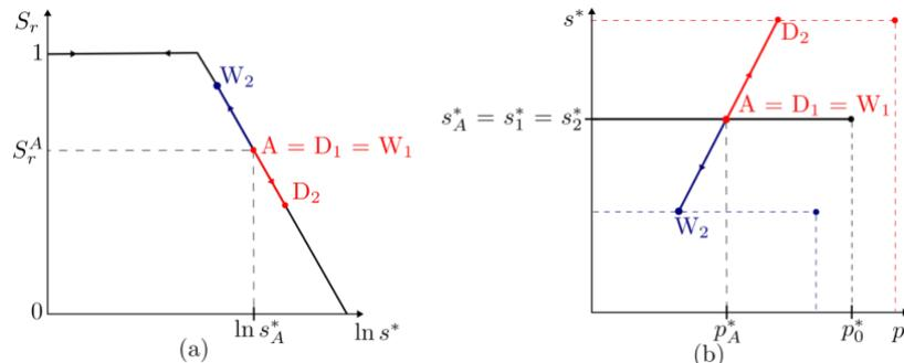
**Figure 3:** The non-hysteretic GCM version for isotropic stress conditions: (a) Typical wetting/drying retention behaviour in the  $S_r: \ln s^*$  plane; (b) Typical DR and WR yielding stress paths in the  $s^*: p^*$  plane.
