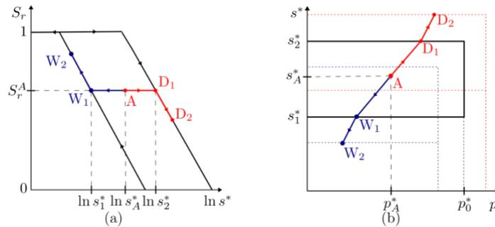
**Figure 2:** The GCM model for isotropic stress conditions: (a) Typical wetting and drying water retention behaviour; (b) Typical wetting and drying paths involving water retention yielding.
