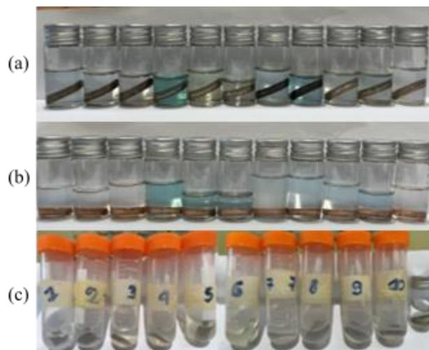
**Figure 3** Physical appearance after 120 hours of (a) copper-nickel, (b) copper and (c) mild steel samples submerged into the desiccant solutions at room temperature (the numbers 1-11 represent the types of desiccant solutions shown in Table 1).
