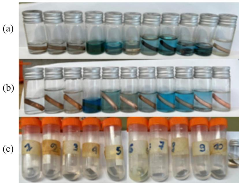
**Figure 4** Physical appearance after 120 hours of (a) copper-nickel, (b) copper and (c) mild steel submerged into the desiccant solutions at  $60\text{ }^\circ\text{C}$  (the numbers 1–11 represent the types of desiccant solutions shown in Table 1).
